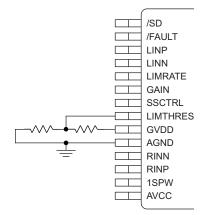
Figure 1. TPA3140D2 LIMTHRES Voltage Divider
