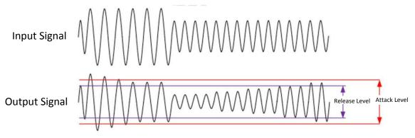
Figure 5. TPA3140D2 AGL Attack/Release Levels
