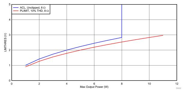
Figure 8. LIMTHRES Voltage vs Output Power with 8- $\Omega$  Load
