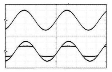
Figure 2. Clipped Power Limiter, PLIMIT
