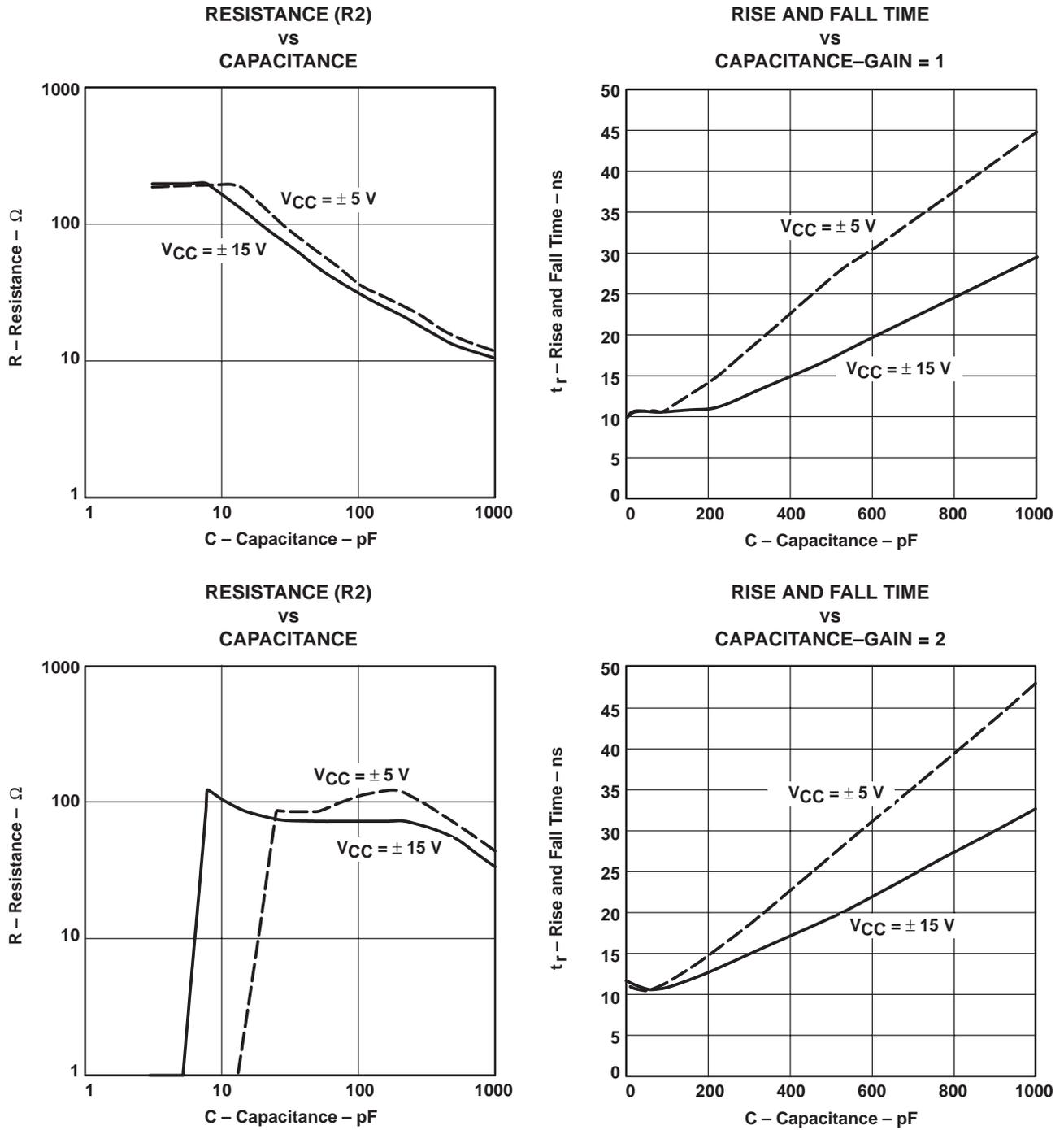
Figure 2. R2 and Rise Time vs Capacitance
