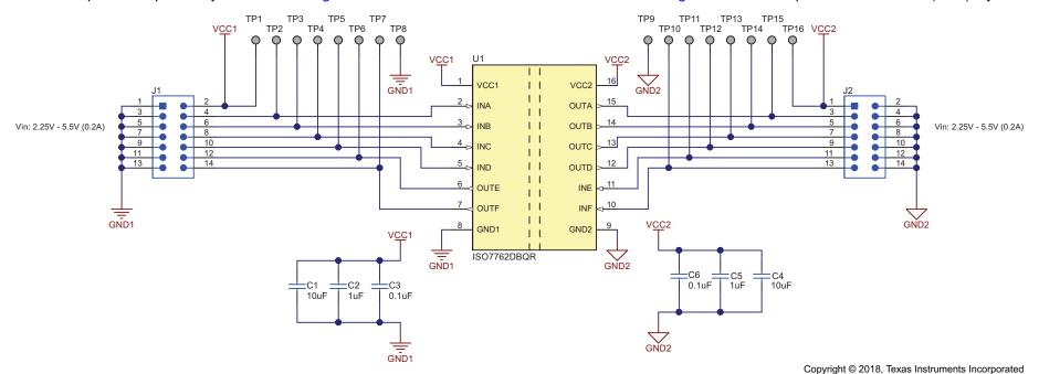
Figure 6. ISO7762DBQEVM Schematic
