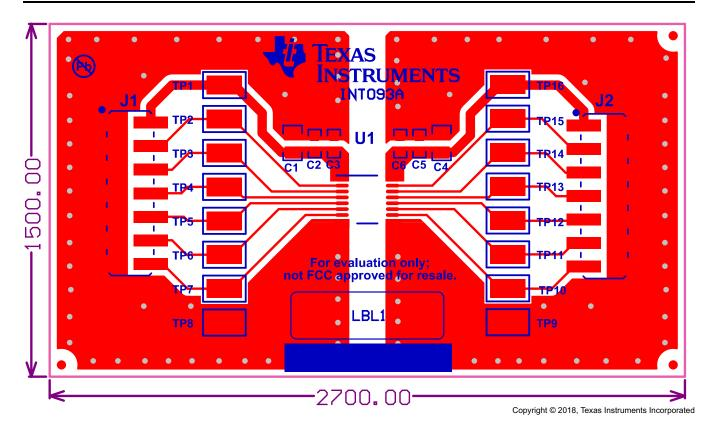
Figure 7. ISO7762DBQEVM PCB Layout
