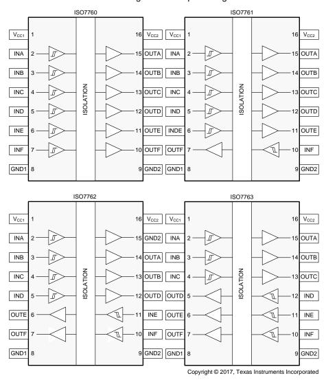
Figure 1. ISO776x Six-Channel Digital Isolator Pin Configurations
