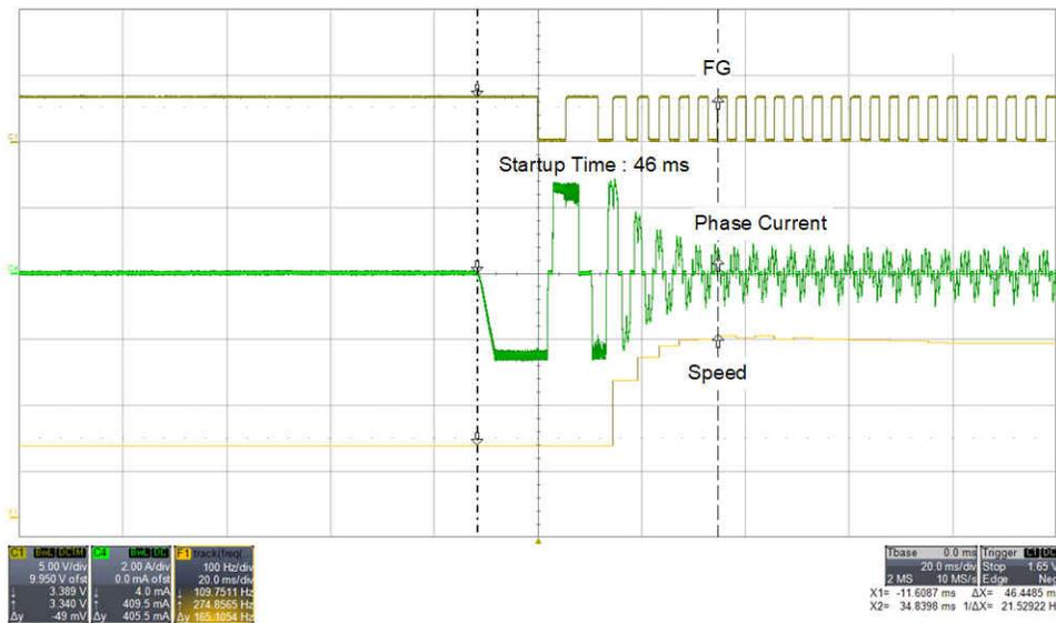
**Figure 2-1. Startup Time Using Align as Motor Startup Method**
