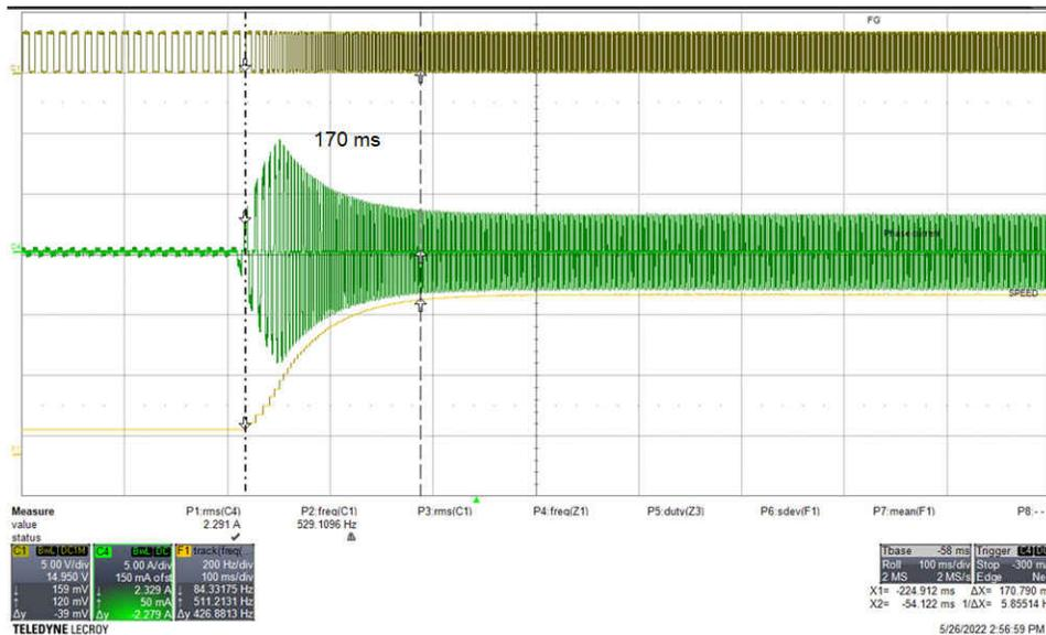
**Figure 2-3. Fast Acceleration**
