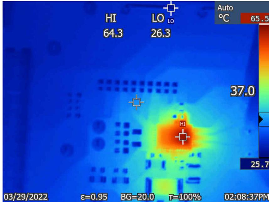
Figure 2-6. Thermal Image of MCT8316A - Lower Case Temperature
