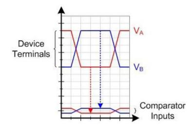
Figure 4-2. Receiver Input-Voltage Attenuation
