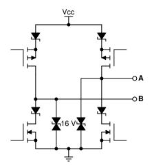
Figure 2-1. Differential Output Driver Structure
