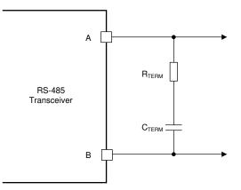
Figure 6-3. AC Termination Network
