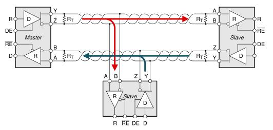
Figure 1-2. Half- and Full-Duplex RS-485 Network Connections
