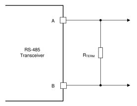
Figure 6-2. Standard Termination Network
