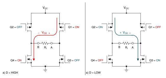
Figure 2-2. RS-485 Output Driver Operation
