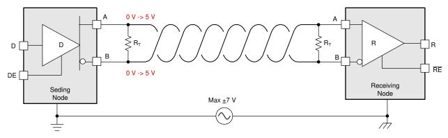
Figure 3-2. Maximum GPD of a Standard RS-485 Transceiver
