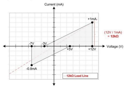
Figure 4-3. RS-485 Receiver Input I-V Characteristic
