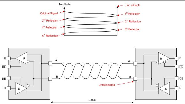
Figure 6-1. Amplitude of Reflection Decay Each Time a Reflection Occurs
