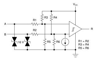
Figure 4-1. Differential Receiver Input Structure
