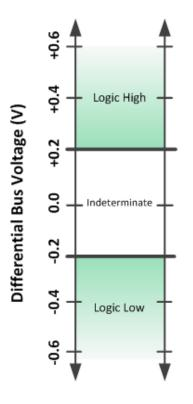
Figure 5-1. RS-485 Receiver Input Thresholds
