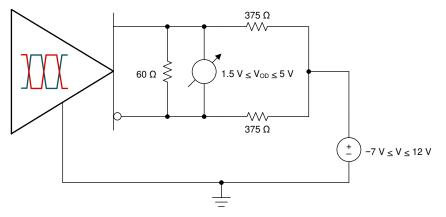
Figure 3-3. RS-485 Driver-Output Test Circuit With Common-Mode Load
