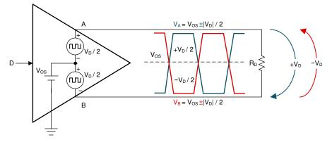
Figure 2-3. RS-485 Driver Output Waveform
