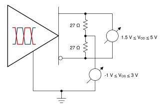
Figure 2-4. RS-485 Output Driver Test Circuit
