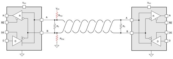
Figure 5-2. Fail-Safe Resistor Placement
