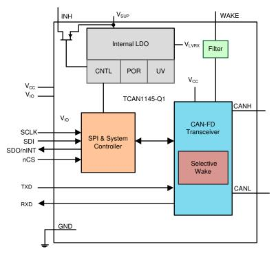
Figure 1-1. Functional Block Diagram
