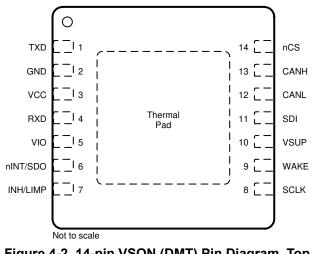
Figure 4-2. 14-pin VSON (DMT) Pin Diagram, Top View
