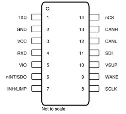
Figure 4-3. 14-pin SOT (DYY) Pin Diagram, Top View
