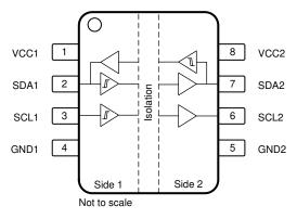
Figure 4-1. Pin Diagram (8-D) Package
