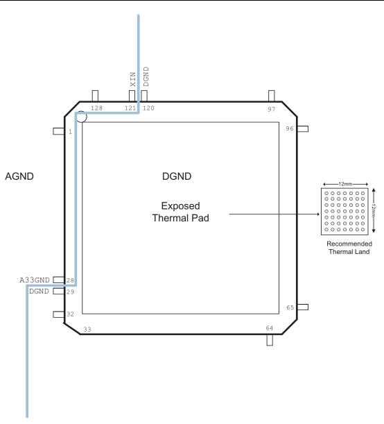
Figure 1. Recommended Split Between Ground Planes
