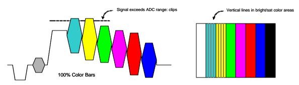
Figure 6. Faint Vertical Lines in 100% Color Bar
