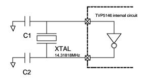
Figure 5. TVP5146 Crystal Circuit
