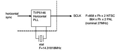
Figure 10. Line-Locked Sampling
