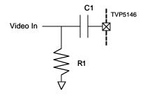
Figure 2. Recommended Analog Input Circuit
