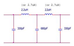
Figure 4. Anti-Aliasing Filter Example Circuit
