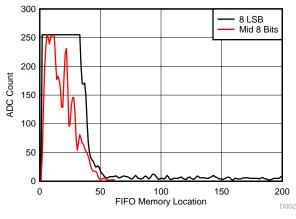
Figure 2. FIFO\_CTRL Comparison for No Object
