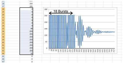
Figure 5. FIFO Data Exported to Excel for Zero-Crossing Analysis
