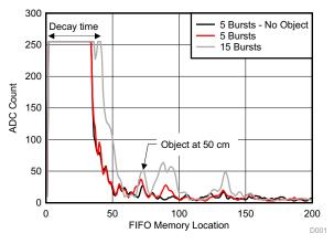
Figure 1. Burst Count Comparison for Object at 50 cm
