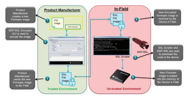
Figure 3: Crypto-Bootloader tools in in-field firmware updates flow
