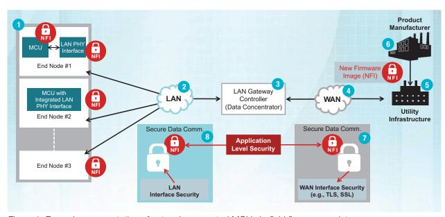
Figure 1: Example representation of network-connected MCUs in-field firmware updates
