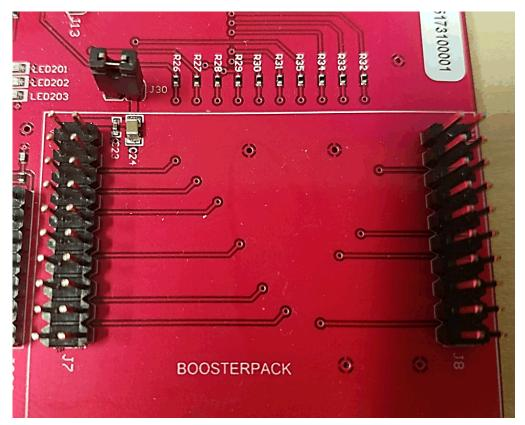
Figure 6. Headers for BoosterPack Plug-in Modules
