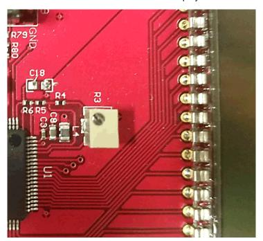
**Figure 12. LCD Contrast Control**
