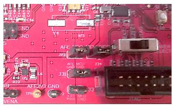
Figure 13. MCU Voltage Source
