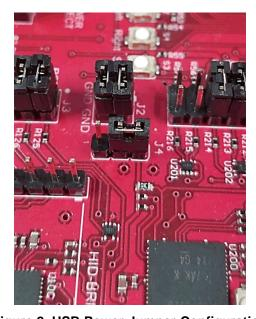
Figure 2. USB Power Jumper Configuration
