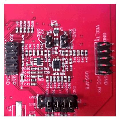
Figure 5. Transducer Header
