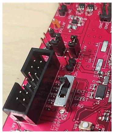
Figure 4. Current Measurement Header
