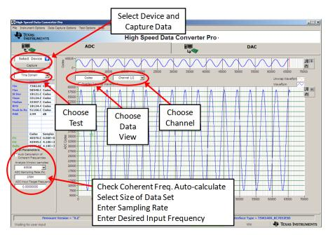
Figure 4. HSDC Pro GUI Main Panel
