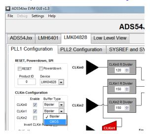
Figure 8. GUI CMOS Selection
