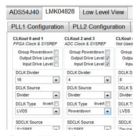
Figure 9. LMK04828 Clock Outputs Tab
