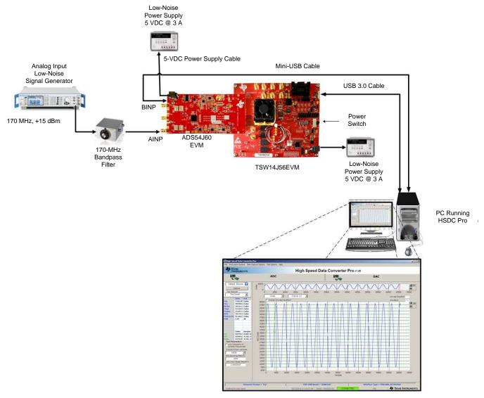
Figure 2. Quick Start Test Setup
