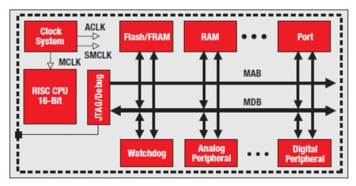
Figure 4. MSP430 MCU for IEC 60730 Applications – Overview of System Architecture
