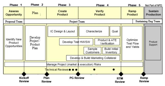
Figure 8. TI Standard MCU QM Development Process
