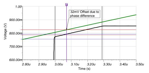
Figure 19. TINA-TI™ Simulation Result—Phase Shift between Input and Sampled Signals
