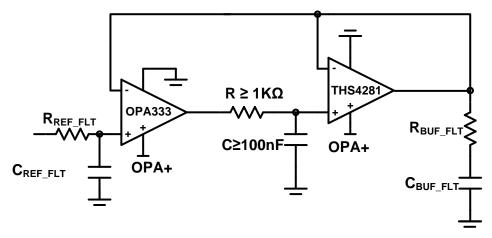
Figure 12. DC-Equivalent Schematic of Reference Buffer
