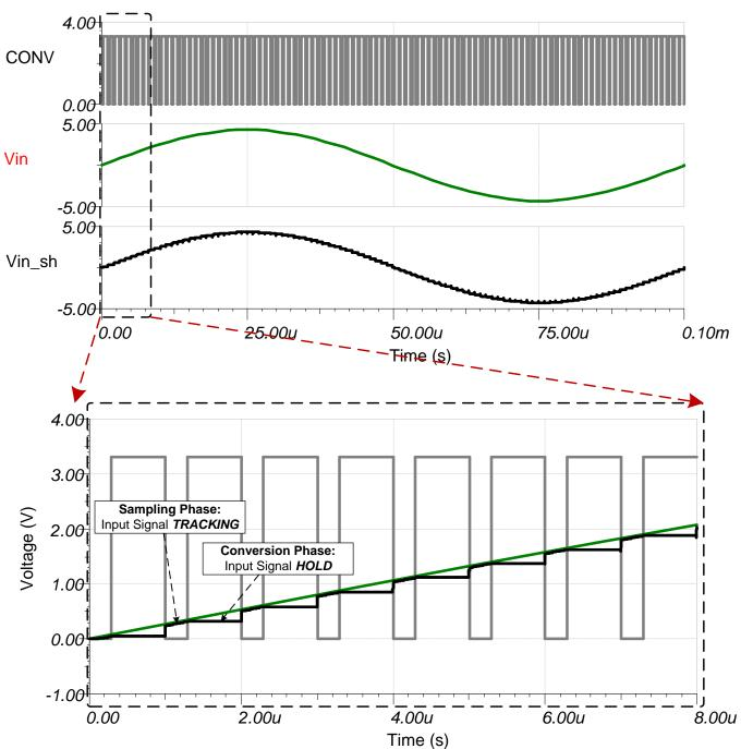
Figure 18. TINA-TI™ Simulation Result—Digitization of Input Sine-Wave Showing ADC Sample-and-Hold
