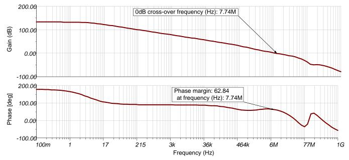
Figure 17. TINA-TI™ Simulation Result—Loop Gain Magnitude and Phase Plot for Input Driver Stability
