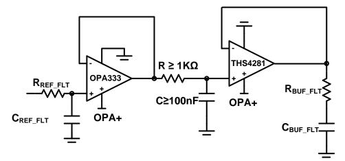
Figure 13. High-Frequency Equivalent Schematic of Reference Buffer Circuit
