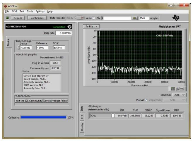
Figure 22. Measurement Data—AC Performance of DAQ Block Using ADCPro™
