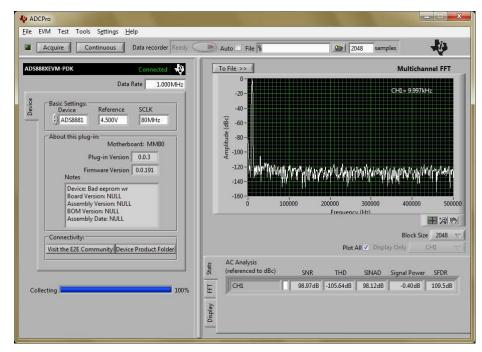
Figure 1. Measurement Data—AC Performance of DAQ Block Using ADCPro™
