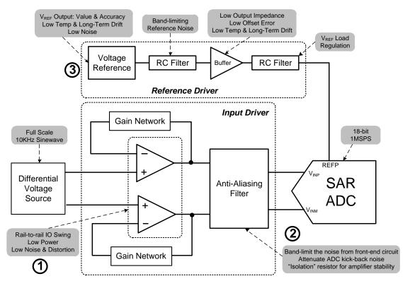
Figure 2. Block Diagram Highlighting Primary Design Criteria for DAQ Block
