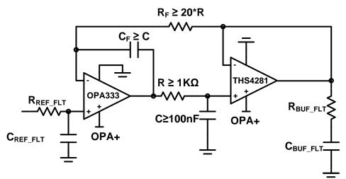
Figure 11. Schematic of Reference Buffer Circuit
