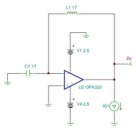
Figure 9. TINA-TI™ Schematic: Measuring Output Impedance of OPA320
