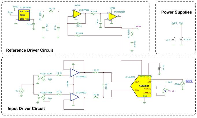
Figure 15. TINA-TI<sup>™</sup> Schematic—Complete DAQ Block
