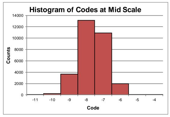
Figure 21. Measurement Data—Histogram Showing DC Noise (Mid-Scale)
