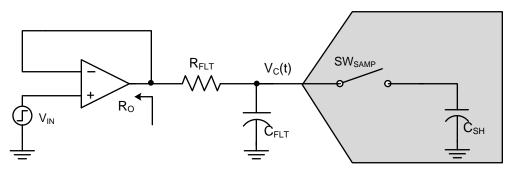
Figure 4. Simplified Schematic of Single-Ended ADC Input Stage
