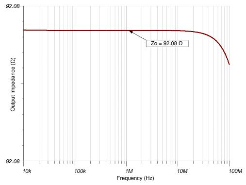
Figure 10. TINA-TI™ Simulation Result: Output Impedance of OPA320
