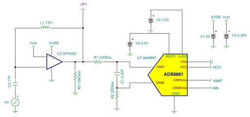
Figure 16. TINA-TI™ Schematic—Checking Input Amplifier Stability
