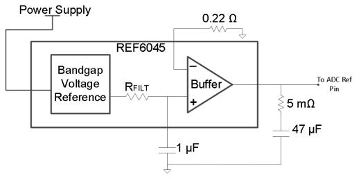
Figure 14. REF6045 Voltage Reference With Integrated Buffer
