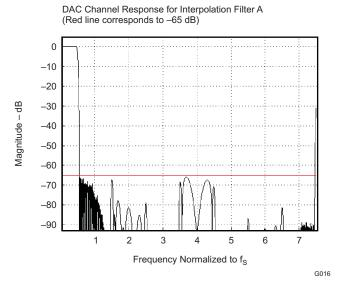
Figure 2-30. DAC Interpolation Filter A, Frequency Response
