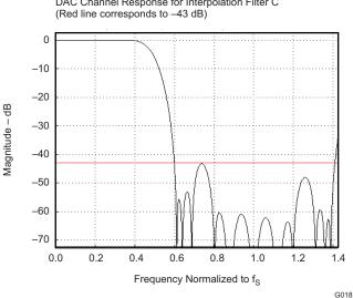
DAC Channel Response for Interpolation Filter C (Red line corresponds to  $-43~\mbox{dB})$
