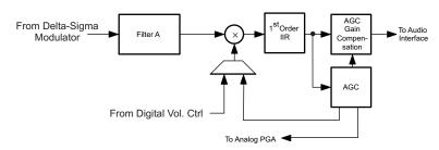
Figure 2-7. Signal Chain for PRB\_R1 and PRB\_R4
