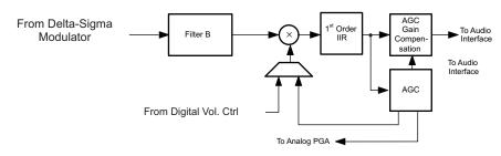
Figure 2-10. Signal Chain for PRB\_R7 and PRB\_R10
