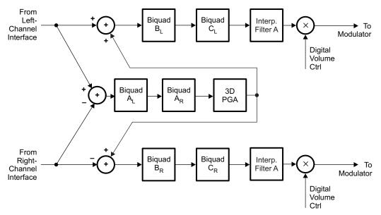
Figure 2-27. Signal Chain for PRB\_P23
