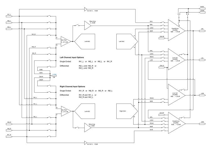
Figure 2-1. Analog Routing Diagram
