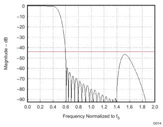
Figure 2-17. ADC Decimation Filter B, Frequency Response
