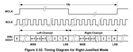
For Right-Justified mode, the number of bit-clocks per frame should be greater than twice the programmed word-length of the data.
