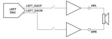
Figure 2-4. Low Power Mono DAC to Differential Headphone
