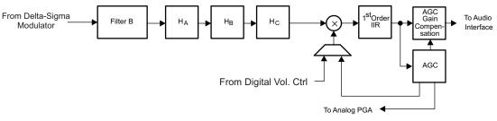
Figure 2-11. Signal Chain for PRB\_R8 and PRB\_R11
