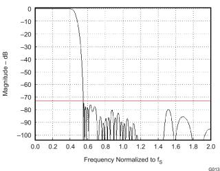
Figure 2-16. ADC Decimation Filter A, Frequency Response
