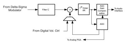
Figure 2-13. Signal Chain for PRB\_R13 and PRB\_R16
