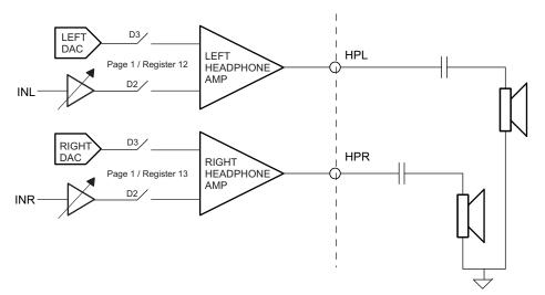
Figure 2-2. Stereo Headphone Configuration
