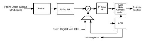
Figure 2-9. Signal Chain for PRB\_R3 and PRB\_R6
