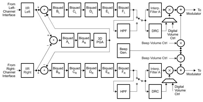
Figure 2-29. Signal Chain for PRB\_P25
