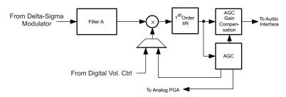
Figure 2-7. Signal Chain for PRB\_R1 and PRB\_R4
