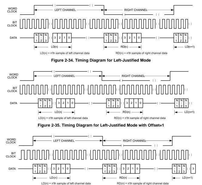
Figure 2-36. Timing Diagram for Left-Justified Mode with Offset=0 and inverted bit clock
