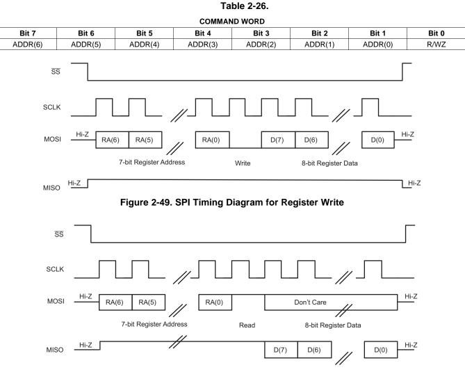
Figure 2-50. SPI Timing Diagram for Register Read
