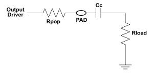
Figure 2-3. Conceptual Circuit for Pop-Free Power-up
