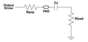
Figure 2-3. Conceptual Circuit for Pop-Free Power-up
