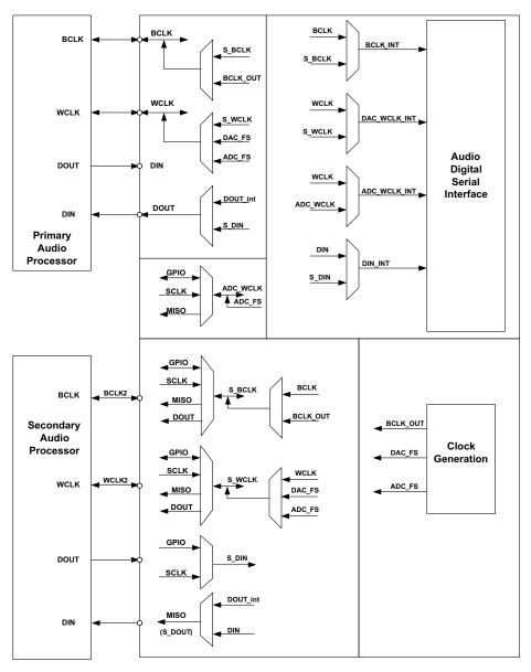
Figure 2-43. Audio Serial Interface Multiplexing
