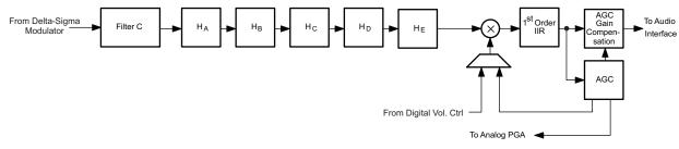
Figure 2-14. Signal Chain for PRB\_R14 and PRB\_R17
