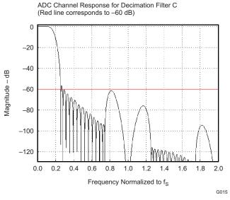
Figure 2-18. ADC Decimation Filter C, Frequency Response
