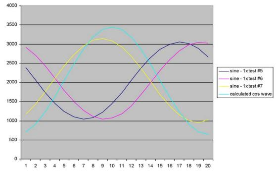
Figure 4. Test #14 Using a sine wave input at 2.8 MHz with a 56 MSPS sample rate. Sine wave amplitude is 1.51V as measured with oscilloscope.
