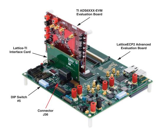
The TI ADS6245EVM board uses jumpers to set various features on the board. The jumpers are located along the left edge of the board when viewed with the silkscreen text readable. The jumper settings should be adjusted to match the following:
