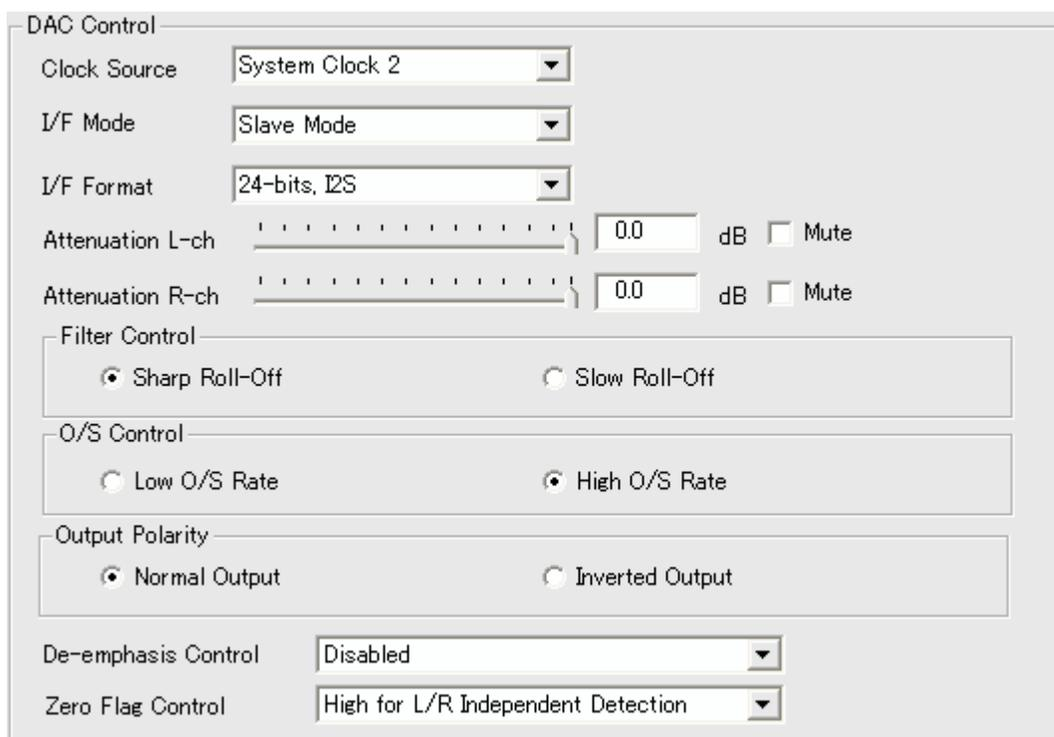
The DAC Control Panel is a software interface for configuring a DAC. It includes the following controls:
