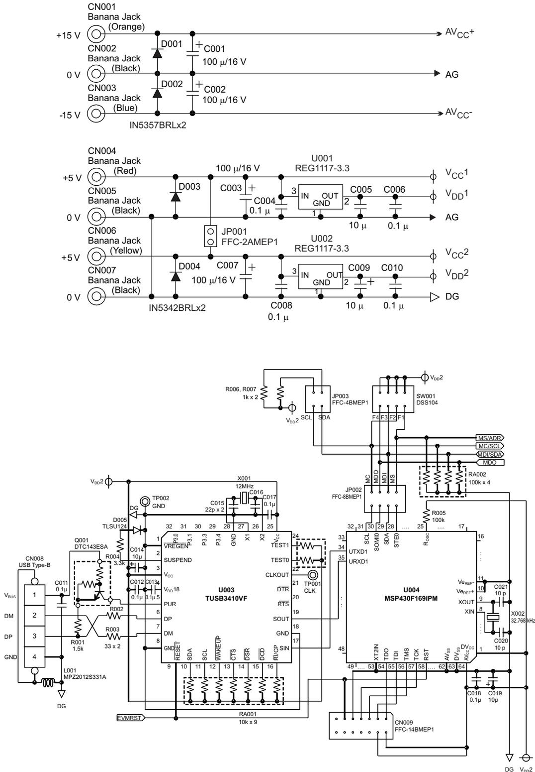
Figure 11. Regulator and Mode Control
