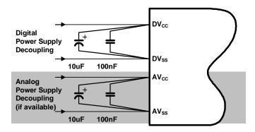
Figure 27-15. ADC10 Grounding and Noise Considerations (external Vref).
