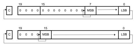
RRC[.W] Rotate Right through carry destination word RRC.B Rotate Right through carry destination byte
