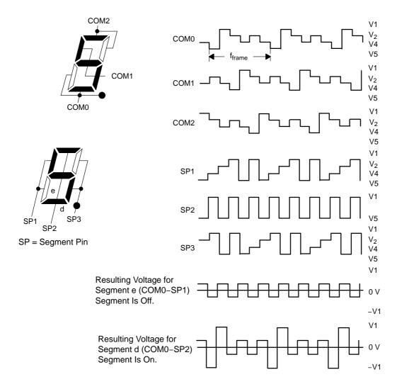
Figure 25–8 shows an example 3-mux LCD, pinout, LCD-to-MSP430 connections, and the resulting segment mapping. This is only an example. Segment mapping in a user's application depends on the LCD pinout and on the MSP430-to-LCD connections.
