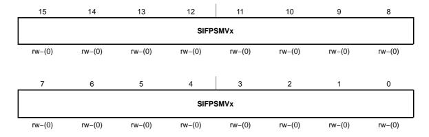
SIFPSMVx Bits SIF PSM vector. These bits are the address for the first state in the PSM state table.
