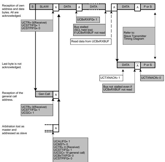
Figure 21–10. I<sup>2</sup>C Slave Receiver Mode
