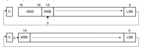
RRUX.A Rotate Right unsigned the 20-bit operand RRUX[.W] Rotate Right unsigned the 16-bit operand RRUX.B Rotate Right unsigned the 8-bit operand
