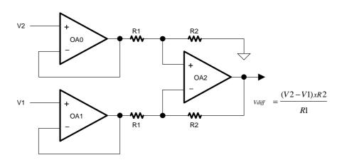
Figure 22–5. Three-Opamp Differential Amplifier OAx Interconnections
