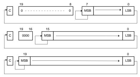
Figure 4–49. Rotate Right Arithmetically RRAX(.B,.A). Non-Register Mode
