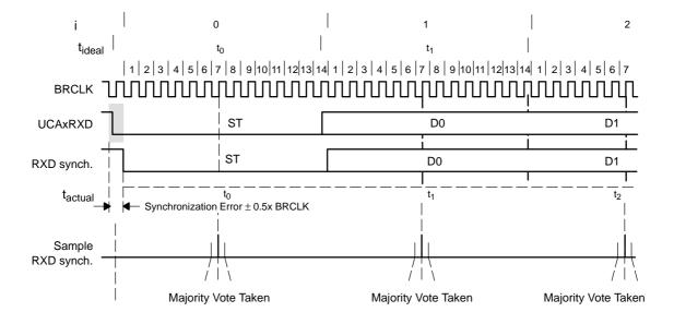
The ideal sampling time t<sub>bit.ideal.RX</sub>[i] is in the middle of a bit period:
