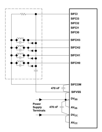
Figure 32-17. LC Sensor Connections For The Envelope Test
