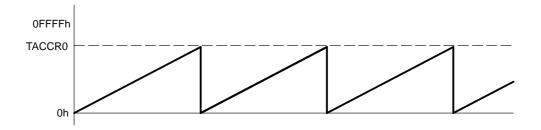
The TACCR0 CCIFG interrupt flag is set when the timer *counts* to the TACCR0 value. The TAIFG interrupt flag is set when the timer *counts* from TACCR0 to zero. Figure 15–3 shows the flag set cycle.
