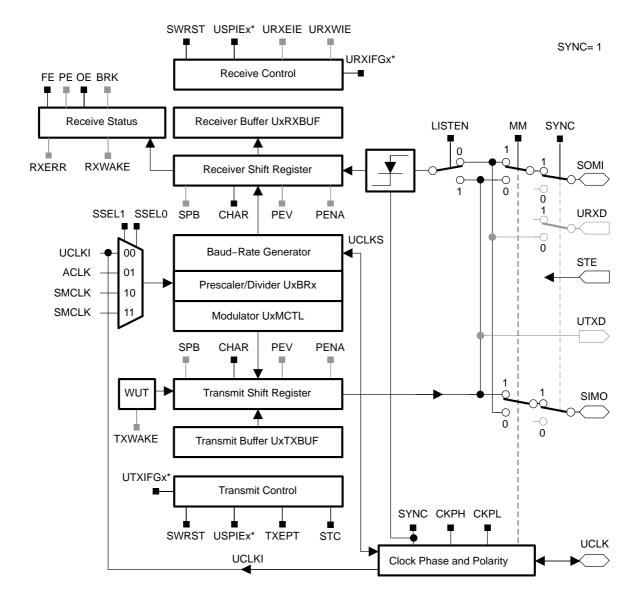
Figure 18-1. USART Block Diagram: SPI Mode
