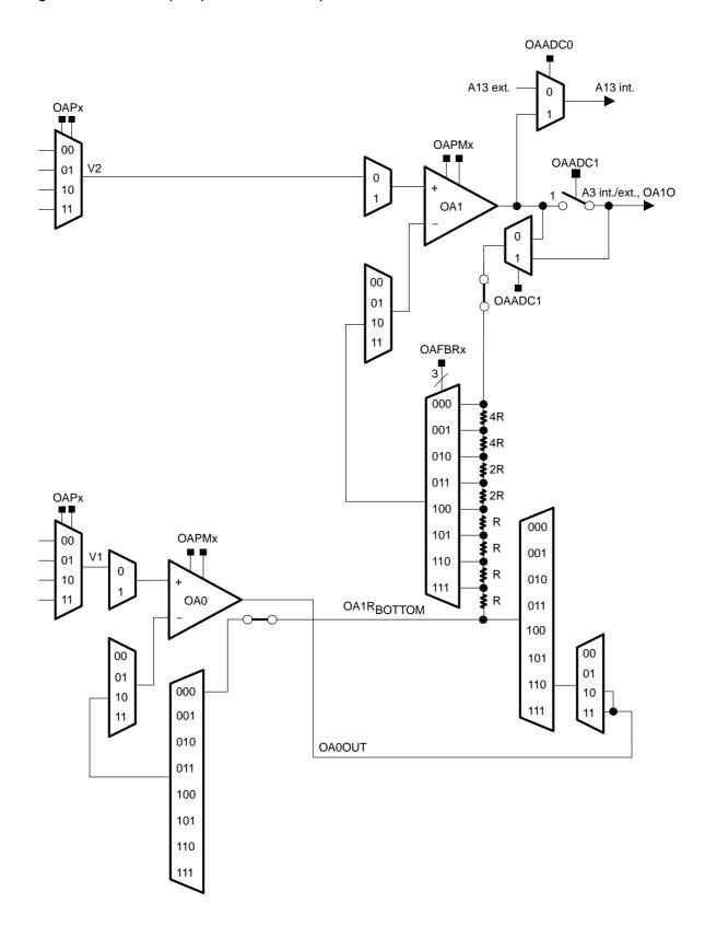
Figure 22–4 shows an example of a three-opamp differential amplifier using OA0, OA1, and OA2. The control register settings are shown in Table 22–4. The gain for the amplifier is selected by the OAFBRx bits of OA0 and OA2. The OAFBRx settings for both OA0 and OA2 must be equal. The gain settings are shown in Table 22–5. The OAx interconnections are shown in Figure 22–5.
