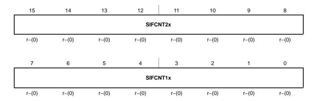
SIFCNT2x Bits SIFCNT2. These bits are the SIFCNT2 counter. SIFCNT2 is reset when 15-8 SIFEN = 0 or if read when SIFCNTRST = 1.
