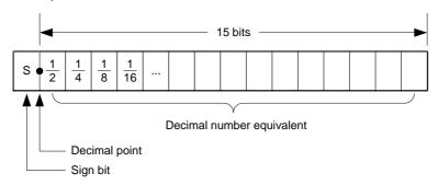
The range can be increased by shifting the decimal point to the right as shown in Figure 9–3. The signed Q14 format with 16 bits gives a range from -2.0 to  $1.999938965 \cong 2.0$ .
