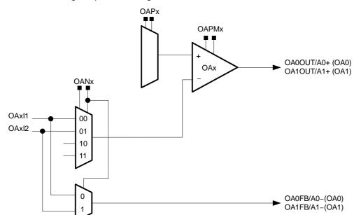
Figure 22–7. Inverting Amplifier Configuration
