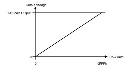
When using 2s compliment data format, the range is shifted such that a DAC12\_xDAT value of 0800h (0080h in 8-bit mode) results in a zero output voltage, 0000h is the mid-scale output voltage, and 07FFh (007Fh for 8-bit mode) is the full-scale voltage output (see Figure 31–5).
