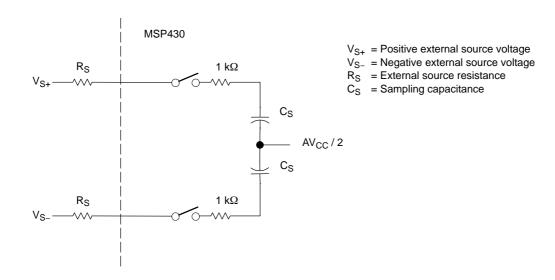
The maximum modulator frequency  $f_M$  may be calculated from the minimum settling time  $t_{Settling}$  of the sampling circuit given by:
