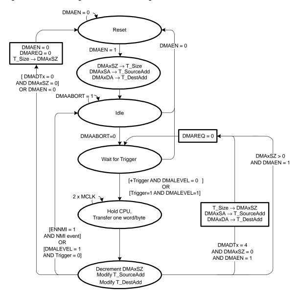
Figure 10-3. DMA Single Transfer State Diagram
