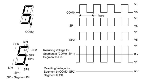
Figure 25–4 shows an example static LCD, pinout, LCD-to-MSP430 connections, and the resulting segment mapping. This is only an example. Segment mapping in a user's application depends on the LCD pinout and on the MSP430-to-LCD connections.
