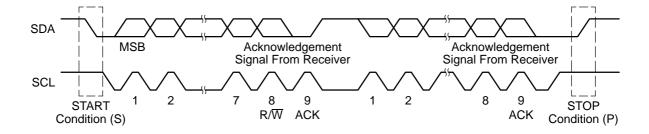
START and STOP conditions are generated by the master and are shown in Figure 21–3. A START condition is a high-to-low transition on the SDA line while SCL is high. A STOP condition is a low-to-high transition on the SDA line while SCL is high. The bus busy bit, UCBBUSY, is set after a START and cleared after a STOP.
