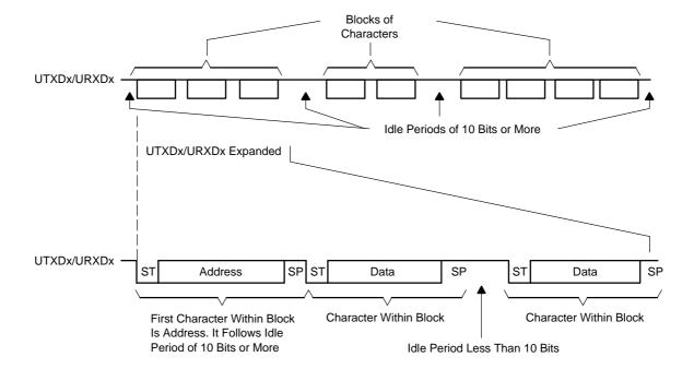
The URXWIE bit is used to control data reception in the idle-line multiprocessor format. When the URXWIE bit is set, all non-address characters are assembled but not transferred into the UxRXBUF, and interrupts are not generated. When an address character is received, the receiver is temporarily activated to transfer the character to UxRXBUF and sets the URXIFGx interrupt flag. Any applicable error flag is also set. The user can then validate the received address.
