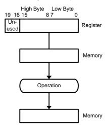
Figure 4-12. Word-Register Operation
