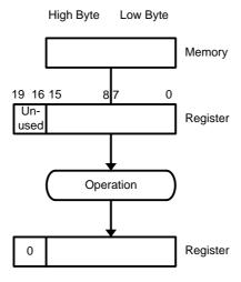
Figure 4–13 and Figure 4–14 show 20-bit address-word handling (.A suffix). The handling is shown for a source register and a destination memory address-word and for a source memory address-word and a destination register.
