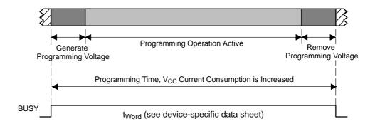
When a byte/word write is executed from RAM, the CPU continues to execute code from RAM. The BUSY bit must be zero before the CPU accesses flash again, otherwise an access violation occurs, ACCVIFG is set, and the write result is unpredictable.
