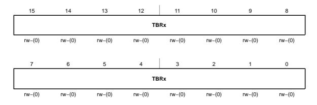
TBRx Bits Timer\_B register. The TBR register is the count of Timer\_B. 15-0
