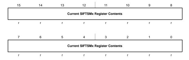
Bits When SIFDEBUG is read, after 02h is written to it, these bits show the TSM output.
