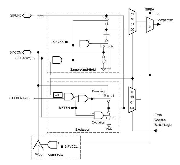
Figure 32-3. Excitation and Sample-And-Hold Circuitry
