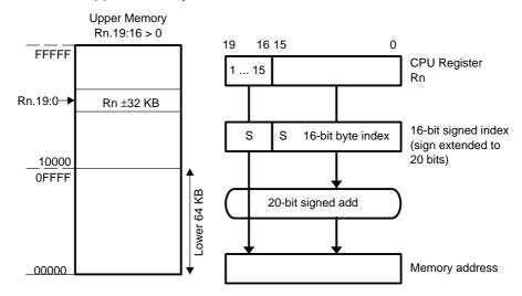
Figure 4-17. Overflow and Underflow for the Indexed Mode
