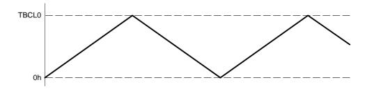
The count direction is latched. This allows the timer to be stopped and then restarted in the same direction it was counting before it was stopped. If this is not desired, the TBCLR bit must be used to clear the direction. The TBCLR bit also clears the TBR value and the clock divider.
