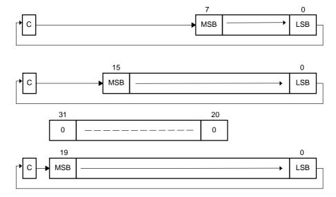
RRUM.A Rotate Right Unsigned the 20-bit CPU register content RRUM[.W] Rotate Right Unsigned the 16-bit CPU register content
