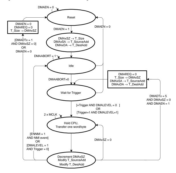
Figure 10-4. DMA Block Transfer State Diagram
