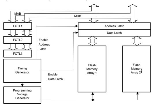
Figure 6-1. Flash Memory Module Block Diagram
