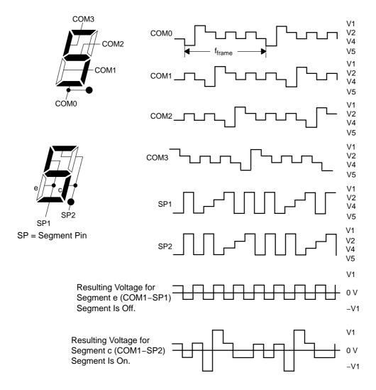
Figure 26–11 shows an example 4-mux LCD, pinout, LCD-to-MSP430 connections, and the resulting segment mapping. This is only an example. Segment mapping in a user's application depends on the LCD pinout and on the MSP430-to-LCD connections.
