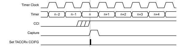
Overflow logic is provided in each capture/compare register to indicate if a second capture was performed before the value from the first capture was read. Bit COV is set when this occurs as shown in Figure 15–11. COV must be reset with software.
