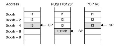
Figure 4–7. PUSHX.A Format on the Stack
