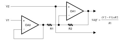
Figure 22–3. Two Opamp Differential Amplifier OAx Interconnections
