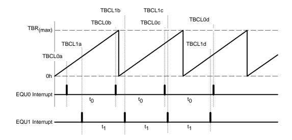
Time intervals can be produced with other modes as well, where TBCL0 is used as the period register. Their handling is more complex since the sum of the old TBCLx data and the new period can be higher than the TBCL0 value. When the sum of the previous TBCLx value plus  $t_{\rm x}$  is greater than the TBCL0 data, TBCL0 + 1 must be subtracted to obtain the correct time interval.
