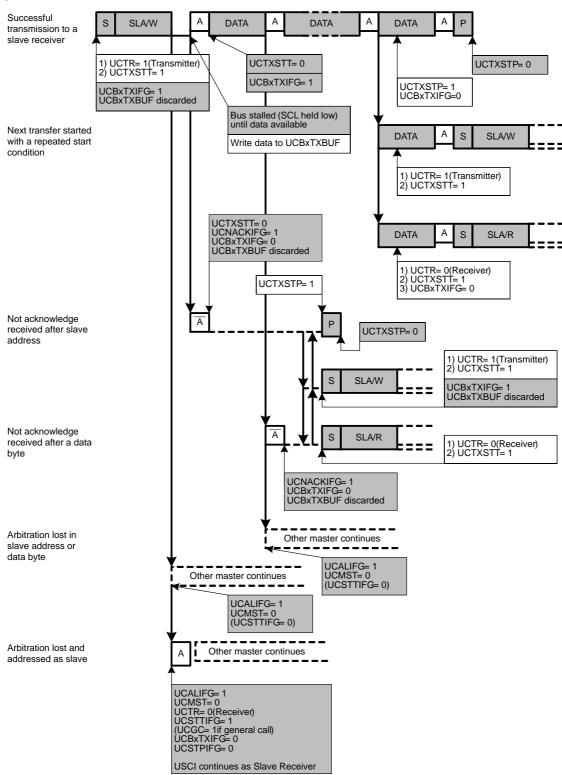
Figure 21–12. I<sup>2</sup>C Master Transmitter Mode
