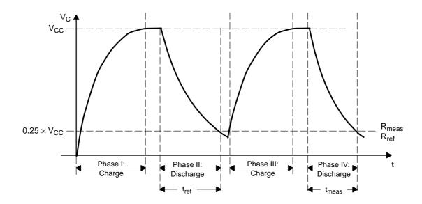
The  $V_{CC}$  voltage and the capacitor value should remain constant during the conversion, but are not critical since they cancel in the ratio:
