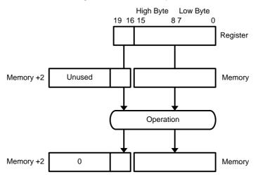
Figure 4–14. Address-Word – Register Operation
