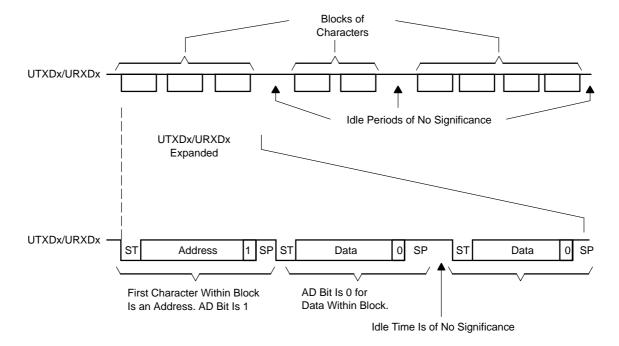
For address transmission in address-bit multiprocessor mode, the address bit of a character can be controlled by writing to the TXWAKE bit. The value of the TXWAKE bit is loaded into the address bit of the character transferred from UxTXBUF to the transmit shift register, automatically clearing the TXWAKE bit. TXWAKE must not be cleared by software. It is cleared by USART hardware after it is transferred to WUT or by setting SWRST.
