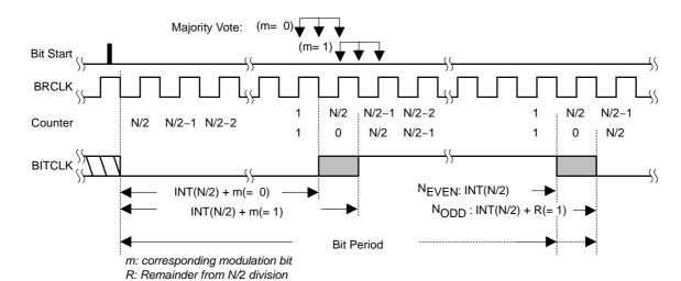
Figure 19–10. BITCLK Baud Rate Timing with UCOS16 = 0
