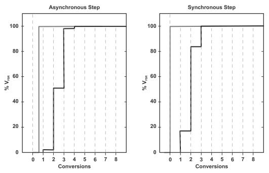
Figure 1. Digital Filter Step Response and Conversion Points
