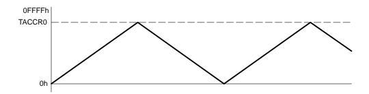
The count direction is latched. This allows the timer to be stopped and then restarted in the same direction it was counting before it was stopped. If this is not desired, the TACLR bit must be set to clear the direction. The TACLR bit also clears the TAR value and the clock divider.
