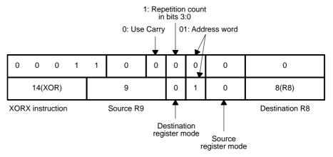
Figure 4–28. Example for an Extended Immediate/Indexed Instruction
