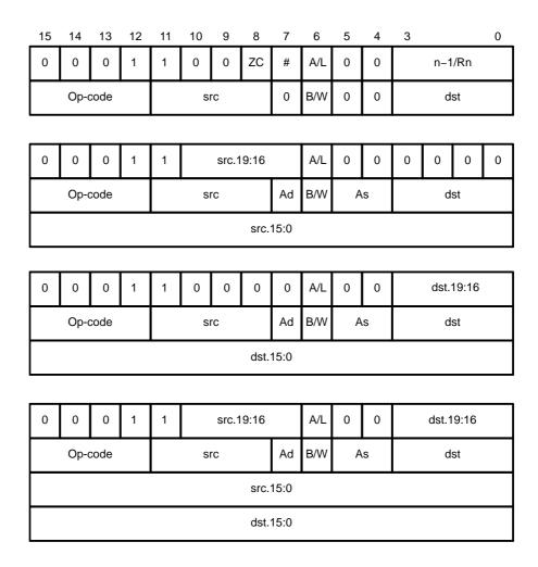
If the 20-bit address of a source or destination operand is located in memory, not in a CPU register, then two words are used for this operand as shown in Figure 4–30.
