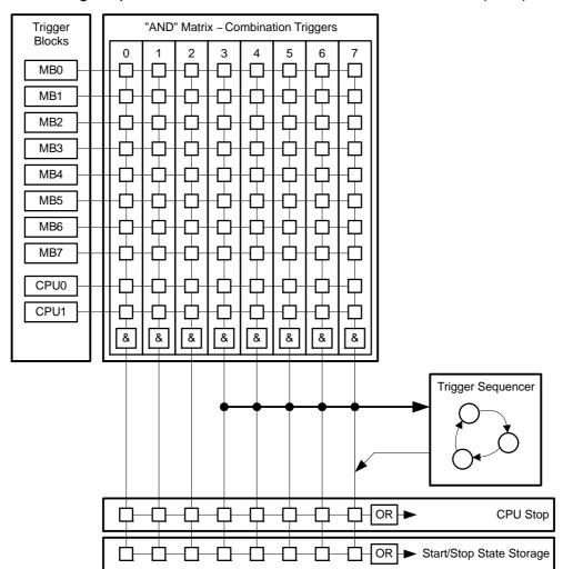
Figure 33–1. Large Implementation of the Embedded Emulation Module (EEM)
