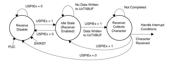
Figure 18–7. SPI Slave Receive-Enable State Diagram
