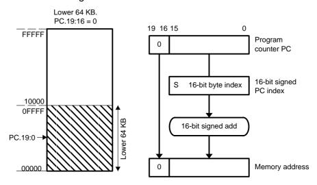
Operation: The signed 16-bit index in the next word after the instruction is added temporarily to the PC. The resulting bits 19:16 are cleared giving a truncated 16-bit memory address, which points to an operand address in the range 00000h, to 0FFFFh. The operand is the content of the addressed memory location.
