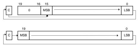
RRCX.A RRCX[.W] RRCX.B Rotate Right through carry the 20-bit operand Rotate Right through carry the 16-bit operand Rotate Right through carry the 8-bit operand
