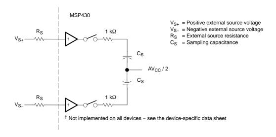
When the buffers are used,  $R_S$  does not affect the sampling frequency  $f_S$ . However, when the buffers are not used or are not present on the device, the maximum modulator frequency  $f_M$  may be calculated from the minimum settling time  $t_{Settling}$  of the sampling circuit given by:
