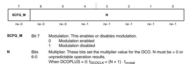
When DCOPLUS = 1:  $f_{DCOCLK} = D \times (N + 1) \cdot f_{crystal}$
