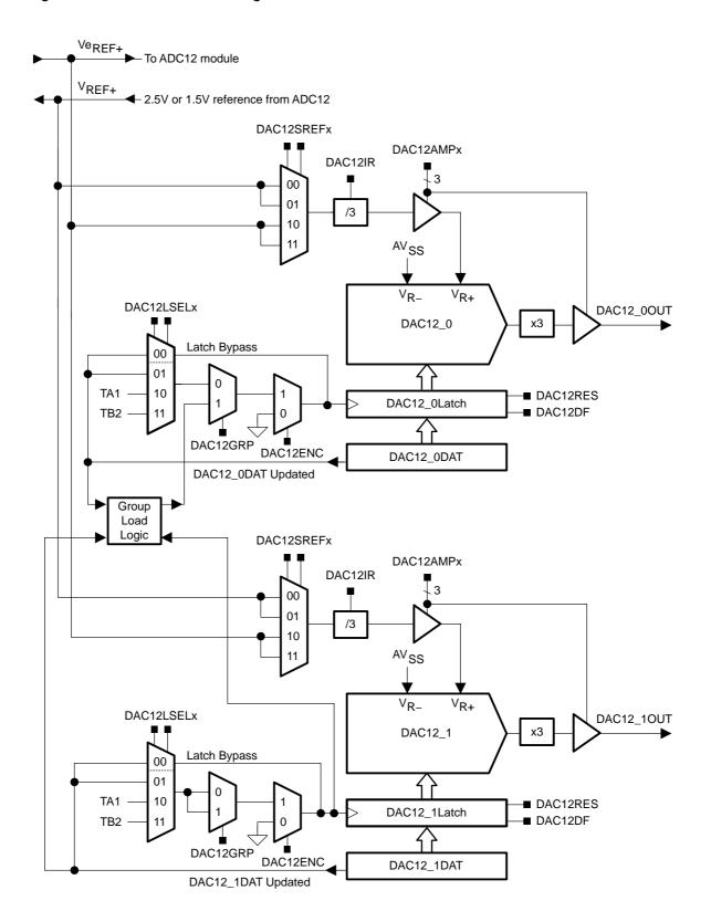
Figure 31–2. DAC12 Block Diagram For MSP430Fx42x0 and MSP430F47x Devices
