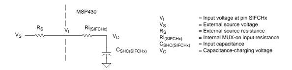
The resistance of the source  $R_S$  and  $Ri_{(SIFCHx)}$  affect  $t_{sample}$ . The following equation can be used to calculate the minimum sampling time  $t_{sample}$  for a 10-bit conversion:
