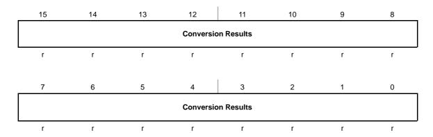
**Conversion** Bits Conversion results. The SD16MEMx register holds the upper or lower 15-0 16-bits of the digital filter output, depending on the SD16LSBACC bit.
