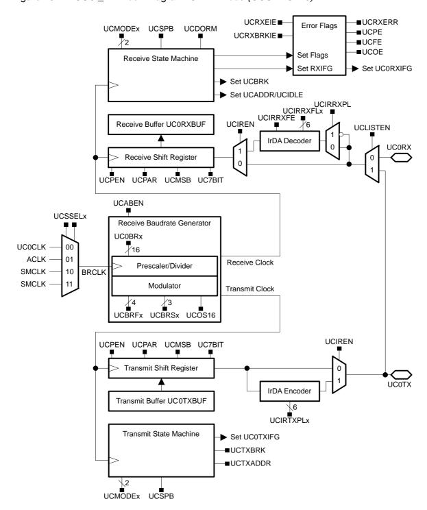
Figure 19–1. USCI\_Ax Block Diagram: UART Mode (UCSYNC = 0)
