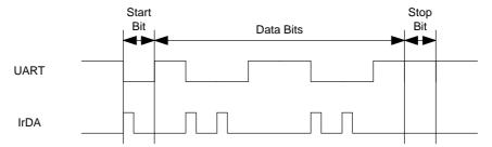
To set the pulse time of 3/16 bit period required by the IrDA standard the BITCLK16 clock is selected with UCIRTXCLK = 1 and the pulse length is set to 6 half clock cycles with UCIRTXPLx = 6 - 1 = 5.
