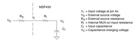
The resistance of the source R<sub>S</sub> and R<sub>I</sub> affect t<sub>sample</sub>. The following equations can be used to calculate the minimum sampling time for a 10-bit conversion.
