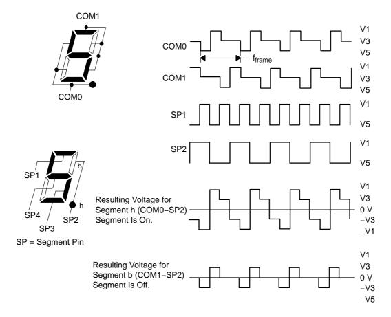
Figure 26–7 shows an example 2-mux LCD, pinout, LCD-to-MSP430 connections, and the resulting segment mapping. This is only an example. Segment mapping in a user's application completely depends on the LCD pinout and on the MSP430-to-LCD connections.
