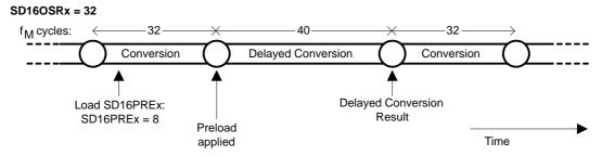
The SD16PREx delay is applied to the beginning of the next conversion cycle after being written. The delay is used on the first conversion after SD16SC is set and on the conversion cycle following each write to SD16PREx. Following conversions are not delayed. After modifying SD16PREx, the next write to SD16PREx should not occur until the next conversion cycle is completed, otherwise the conversion results may be incorrect.
