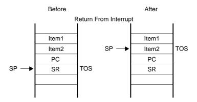
Interrupt nesting is enabled if the GIE bit is set inside an interrupt service routine. When interrupt nesting is enabled, any interrupt occurring during an interrupt service routine will interrupt the routine, regardless of the interrupt priorities.
