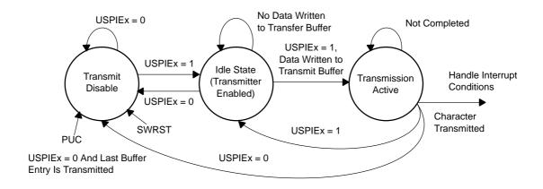
Figure 18-5. Slave Transmit Enable State Diagram
