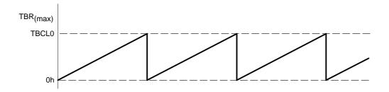
The TBCCR0 CCIFG interrupt flag is set when the timer *counts* to the TBCL0 value. The TBIFG interrupt flag is set when the timer *counts* from TBCL0 to zero. Figure 15–3 shows the flag set cycle.
