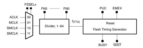
The flash timing generator can be sourced from ACLK, SMCLK, or MCLK. The selected clock source should be divided using the FNx bits to meet the frequency requirements for  $f_{FTG}$ . If the  $f_{FTG}$  frequency deviates from the specification during the write or erase operation, the result of the write or erase may be unpredictable, or the flash memory may be stressed above the limits of reliable operation.
