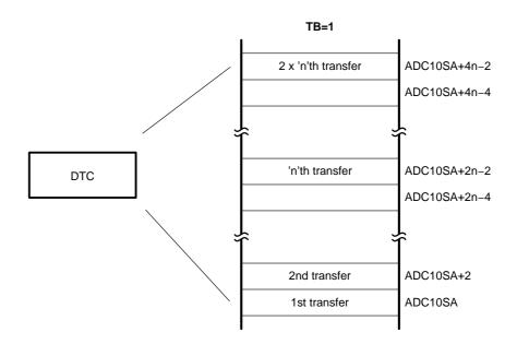
The internal address pointer is initially equal to ADC10SA and the internal transfer counter is initially equal to 'n'. The internal pointer and counter are not visible to software. The DTC transfers the word-value of ADC10MEM to the address pointer ADC10SA. After each DTC transfer the internal address pointer is incremented by two and the internal transfer counter is decremented by one.
