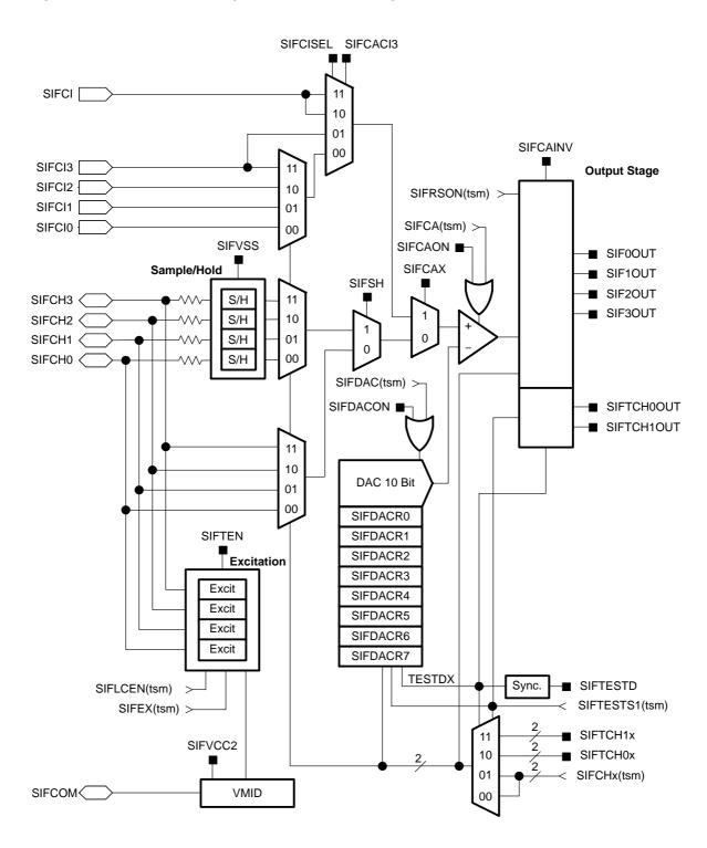
Figure 32-2. Scan IF Analog Front End Block Diagram
