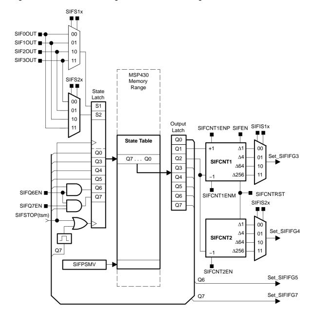
Figure 32-11. Scan IF Processing State Machine Block Diagram
