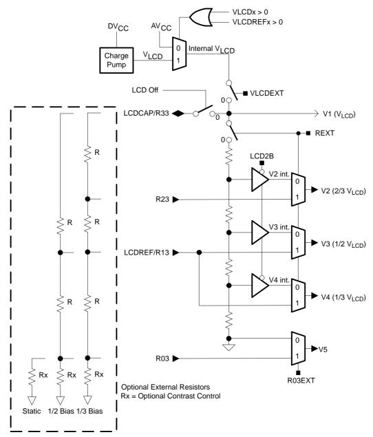
The internal bias generator supports 1/2 bias LCDs when LCD2B = 1, and 1/3 bias LCDs when LCD2B = 0 in 2-mux, 3-mux, and 4-mux modes. In static mode, the internal divider is disabled.
