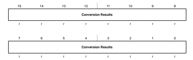
**Conversion** Bits Conversion Results. The SD16MEMx register holds the upper or lower Result 15-0 16-bits of the digital filter output, depending on the SD16LSBACC bit.
