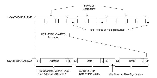
Figure 19–4. Address-Bit Multiprocessor Format
