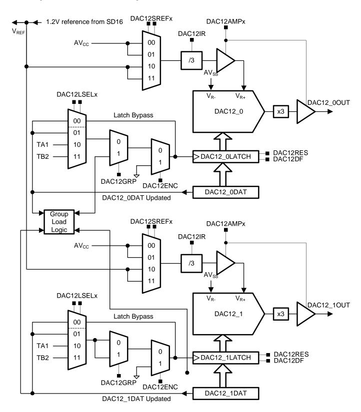
Figure 31-3. DAC12 Block Diagram For MSP430FG47x Devices
