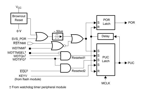
A POR is a device reset. A POR is only generated by the following three events:
