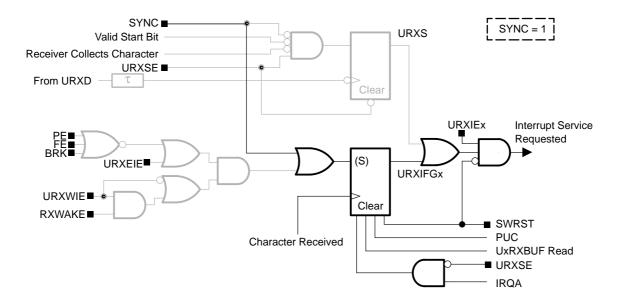
Figure 18–12. Receive Interrupt State Diagram
