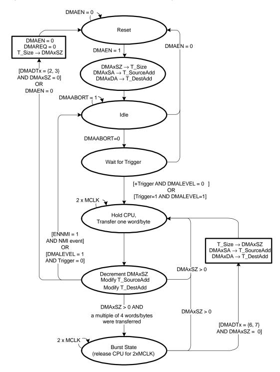
Figure 10-5. DMA Burst-Block Transfer State Diagram
