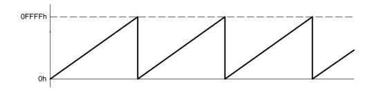
The TAIFG interrupt flag is set when the timer *counts* from 0FFFFh to zero. Figure 15–5 shows the flag set cycle.
