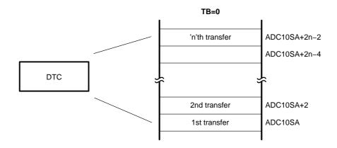
The internal address pointer is initially equal to ADC10SA and the internal transfer counter is initially equal to 'n'. The internal pointer and counter are not visible to software. The DTC transfers the word-value of ADC10MEM to the address pointer ADC10SA. After each DTC transfer, the internal address pointer is incremented by two and the internal transfer counter is decremented by one.
