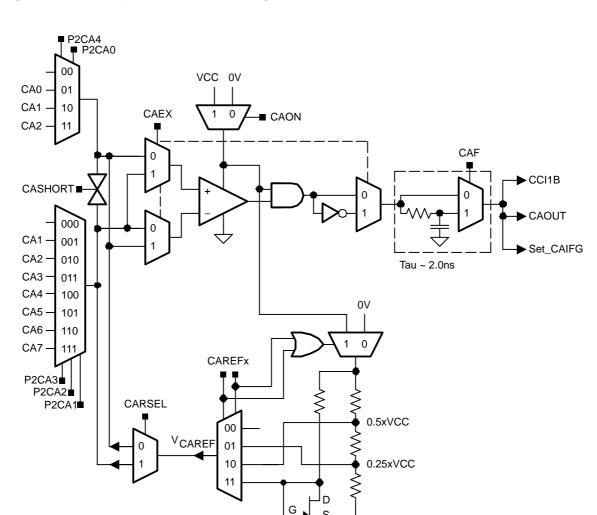
Figure 24–1. Comparator\_A+ Block Diagram
