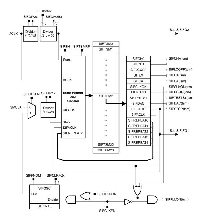
Figure 32-8. Timing State Machine Block Diagram
