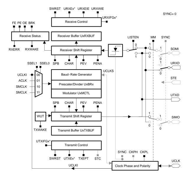
Figure 17-1. USART Block Diagram: UART Mode
