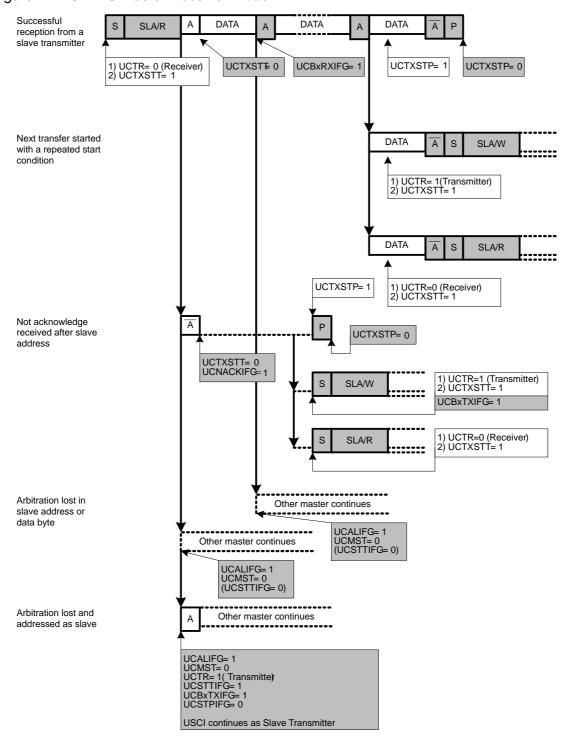
Figure 21–13. I<sup>2</sup>C Master Receiver Mode
