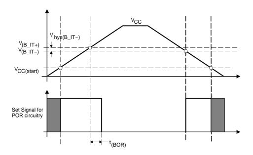
As the  $V_{(B\_IT\_)}$  level is significantly above the  $V_{(MIN)}$  level of the POR circuit, the BOR provides a reset for power failures where  $V_{CC}$  does not fall below  $V_{(MIN)}$ . See the device-specific data sheet for parameters.
