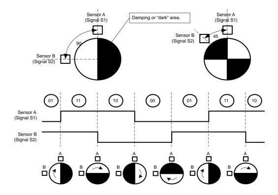
Quadrature decoding requires knowing the previous quadrature pair S1 and S2, as well as the current pair. Comparing these two pairs will tell the direction of the rotation. For example, if the current pair is 00 it can change to 01 or 10, depending on direction. Any other change in the signal pair would represent an error as shown in Figure 32–20.
