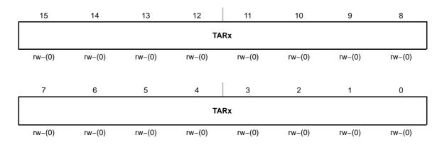
TARx Bits Timer\_A register. The TAR register is the count of Timer\_A.
