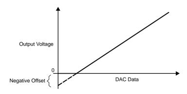
When the output amplifier has a positive offset, a digital input of zero does not result in a zero output voltage. The DAC12 output voltage reaches the maximum output level before the DAC12 data reaches the maximum code (see Figure 31–7).
