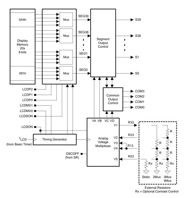
Figure 25–1. LCD Controller Block Diagram
