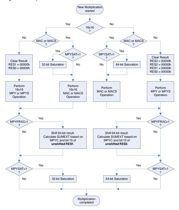
Given the separation in processing of 16-bit operations (32-bit results) and 32-bit operations (64-bit results) by the module, it is important to understand the implications when using MAC/MACS operations and mixing 16-bit operands/results with 32-bit operands/results. User software must address these points during usage when mixing these operations. The following code illustrates the issue.
