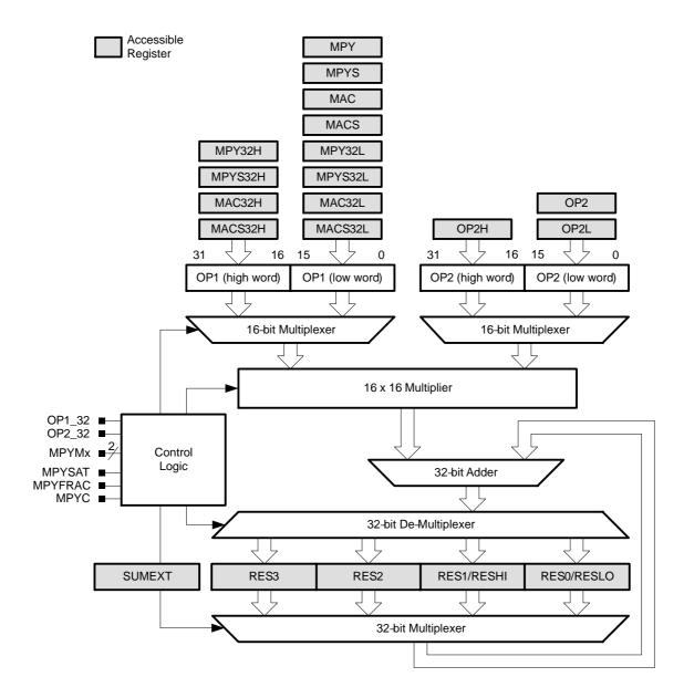
Figure 9-1. 32-Bit Hardware Multiplier Block Diagram
