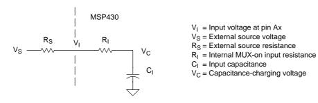
The resistance of the source  $R_S$  and  $R_I$  affect  $t_{sample}$ . The following equation can be used to calculate the minimum sampling time  $t_{sample}$  for a 12-bit conversion:
