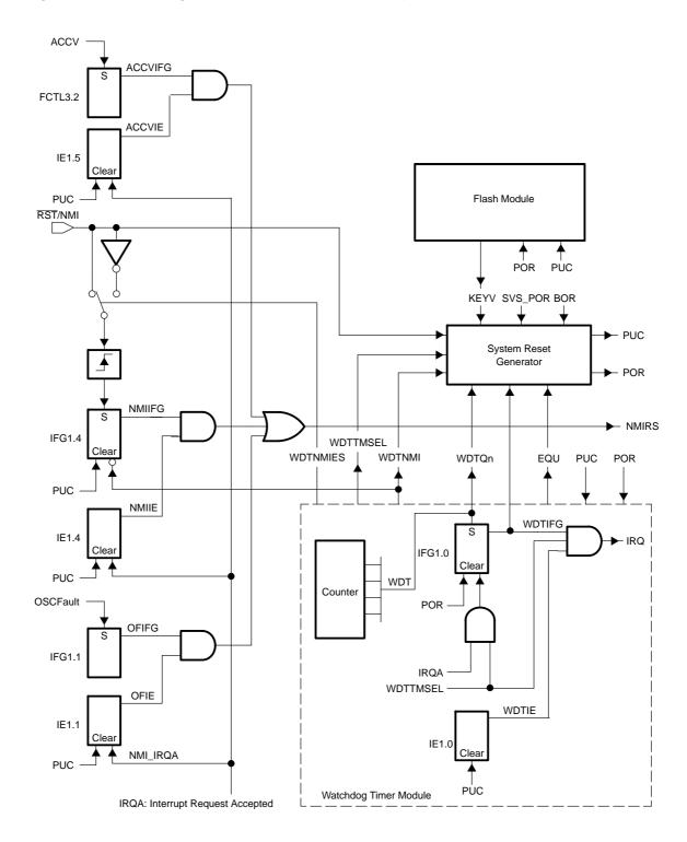
Figure 2-4. Block Diagram of (Non)-Maskable Interrupt Sources
