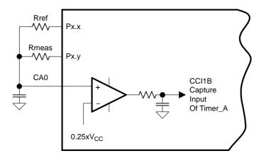
The MSP430 resources used to calculate the temperature sensed by Rmeas are:
