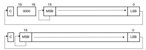
RRAX.A RRAX[.W] RRAX.B Rotate Right Arithmetically the 20-bit operand Rotate Right Arithmetically the 16-bit operand Rotate Right Arithmetically the 8-bit operand
