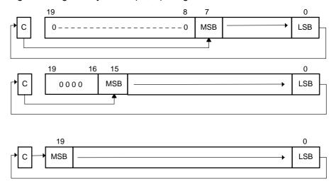
Figure 4-52. Rotate Right Through Carry RRCX(.B,.A). Non-Register Mode
