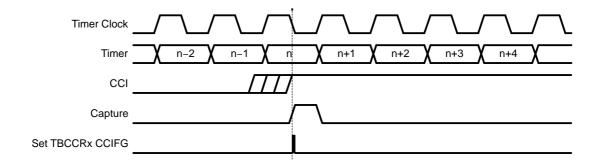
Overflow logic is provided in each capture/compare register to indicate if a second capture was performed before the value from the first capture was read. Bit COV is set when this occurs as shown in Figure 16–11. COV must be reset with software.
