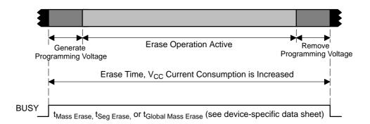
A dummy write to an address not in the range to be erased does not start the erase cycle, does not affect the flash memory, and is not flagged in any way. This errant dummy write is ignored.
