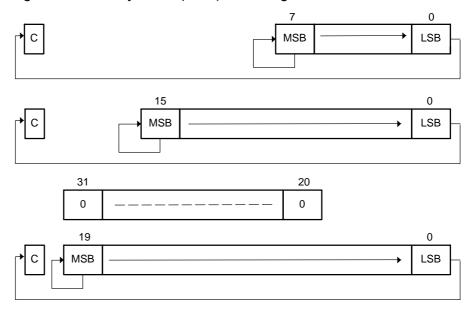
RRCM.A Rotate Right through carry the 20-bit CPU register content RRCM[.W] Rotate Right through carry the 16-bit CPU register content
