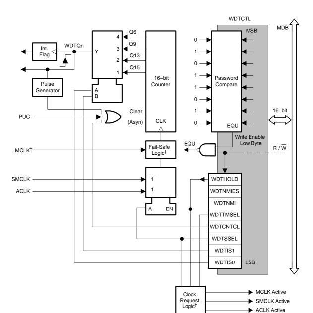
Figure 12-1. Watchdog Timer Block Diagram
