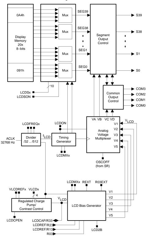
Figure 26–1. LCD\_A Controller Block Diagram
