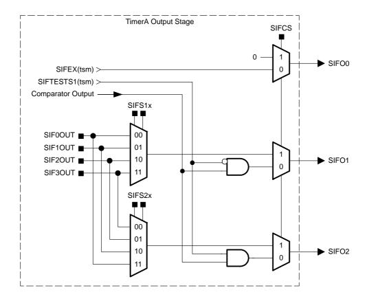
When SIFCS = 0, the SIFEX(tsm) signal and the comparator output can be selected as inputs to different Timer1\_A5 capture/compare registers. This can be used to measure the time between excitation of a sensor and the last oscillation that passes through the comparator or to perform a slope A/D conversion.
