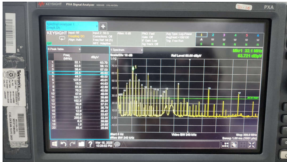
Figure 6-5. Conducted Noise at Vcore on MSPM0L
