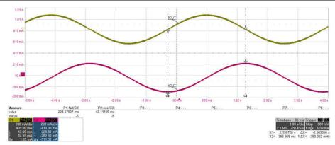
Figure 4-5. Coil Current I-AOUT, I-BOUT for 1/128 Step Mode, 100 PPS
