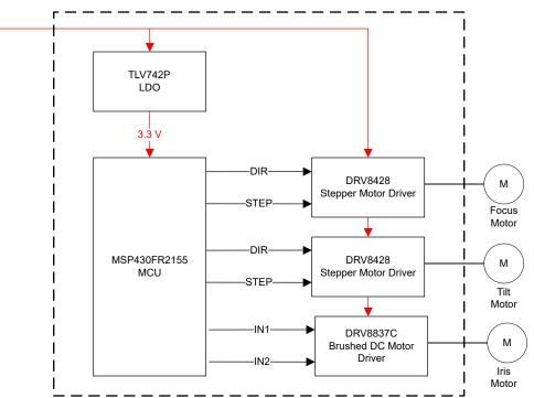
Figure 2-1. Block Diagram of Motor Module
