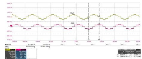
Figure 4-3, Figure 4-4, and Figure 4-5 show the coils currents (I-AOUT, I-BOUT) for different stepping modes.
