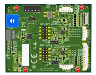
Figure 2-2. Motor Module PCB
