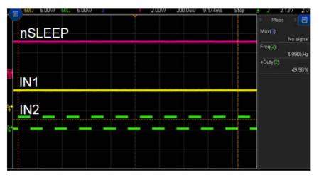
Figure 4-8. Inputs to Motor Driver: nSLEEP, IN1, IN2
