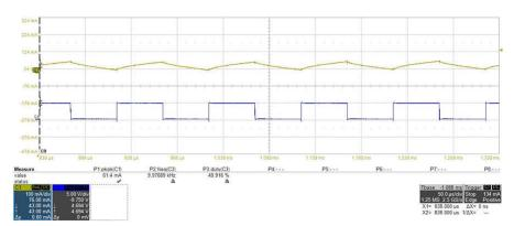
Figure 4-9. Voltage and Current, 50% Duty Cycle, 10 kHz, Reverse Direction
