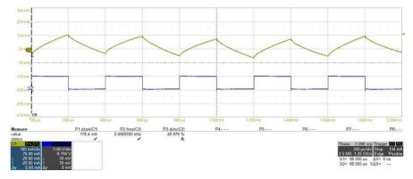
Figure 4-11. Voltage and Current, 50% Duty Cycle, 2.5 kHz, Reverse Direction
