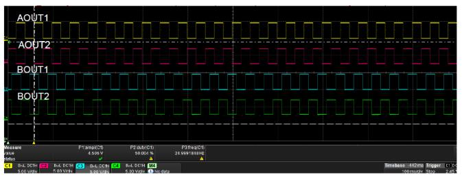
Figure 4-2. Voltage Outputs at No-Load AOUT1, AOUT2, BOUT1, BOUT2 for Full-Step Mode, 100 PPS
