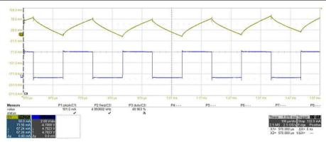
Figure 4-10. Voltage and Current, 50% Duty Cycle, 5 kHz, Reverse Direction
