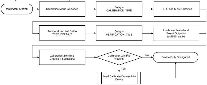
Figure 2-1. Factory Test Calibration Process
