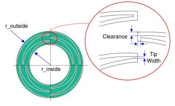
Figure 7. Wheel Radius and Clearance
