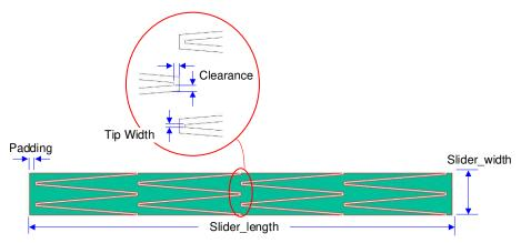
Figure 5. Slider Sensor Clearance
