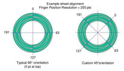
Figure 8. Wheel Orientation
