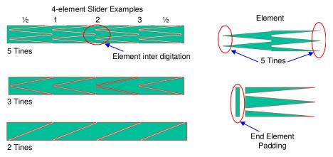
Figure 4. Slider Sensor Elements
