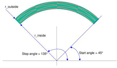
Figure 9. Curved Slider Dimensions
