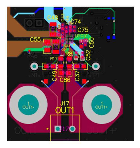
Figure 1-10. OUT\_P, OUT\_N, BST\_P and BST\_N Pins Connections
