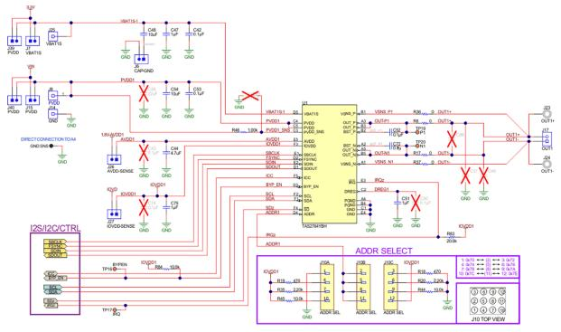
Figure 3-1. TAS2764 Schematic (Sheet 1 of 2)
