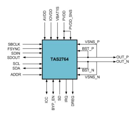
Figure 1-1. TAS2764 Block Diagram
