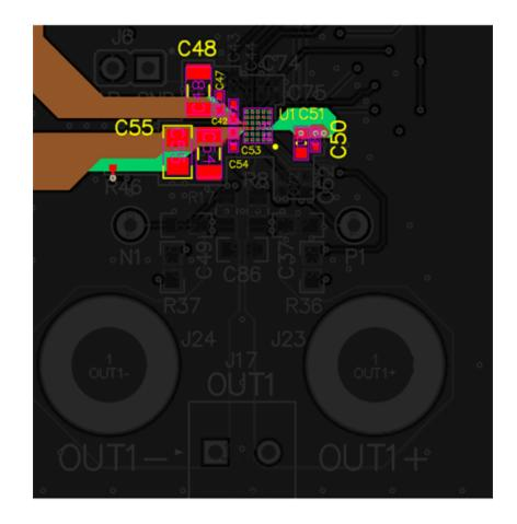
Figure 1-7. PVDD Pin Connection
