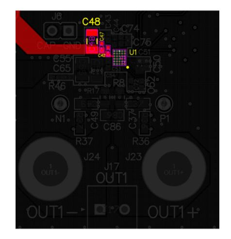
Figure 1-5. VBAT1S Pin Connection
