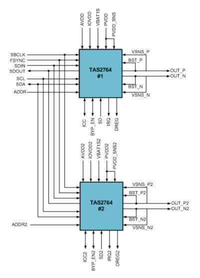
Figure 2-1. TAS2764 Block Diagram (Stereo)
