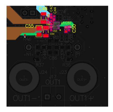
Figure 1-8. AVDD Pin Connection
