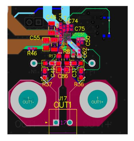
Figure 1-11. VSNS\_P, VSNS\_N and PVDD\_SNS Pins Connections
