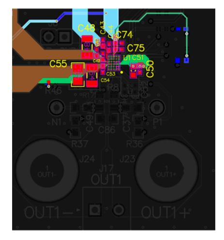
Figure 1-9. IOVDD Pin Connection
