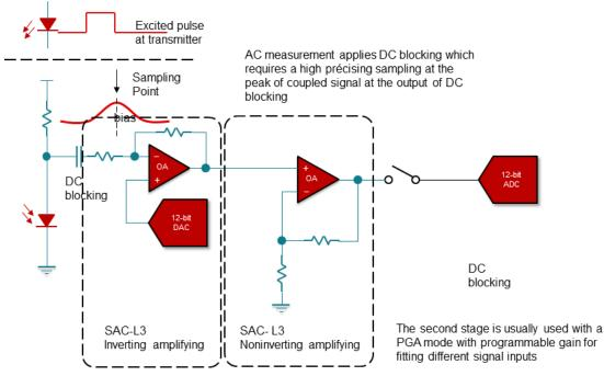
Figure 1. Block Diagram Showing AC Measurement in a Smoke Detector Application Using the MSP430 Smart Analog Combo
