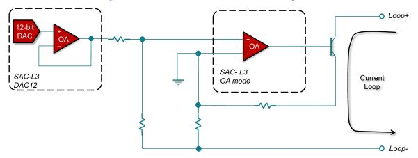
Figure 5. Block Diagram of a Current-Loop Transmitter Using the MSP430 Smart Analog Combo
