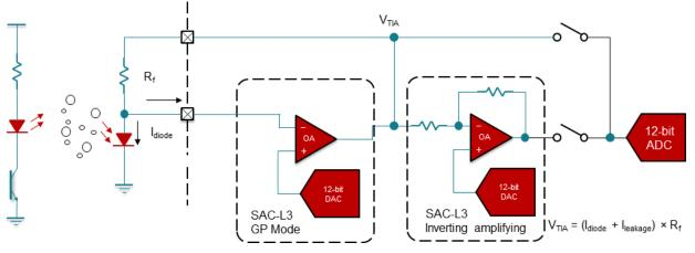
Figure 3. Block Diagram of a Gas Detector Using the MSP430 Smart Analog Combo
