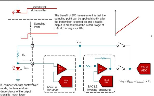
Figure 2. Block Diagram Showing DC Measurement in a Smoke Detector Application Using the MSP430 Smart Analog Combo
