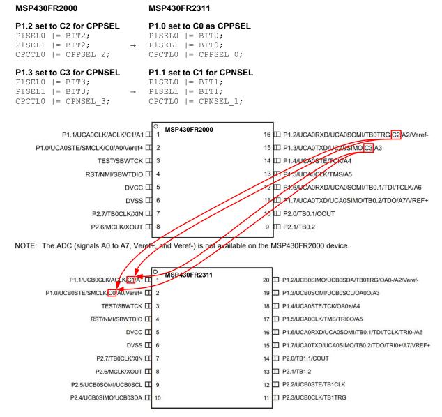
**Figure 3. Comparator Signals**
