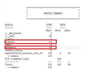
Figure 15. Global Variable Zero-initialization in IAR
