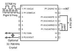
Figure 1. Programmable Clock Source I/Os
