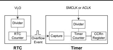
Figure 3. Peripherals Used for VLO Calibration
