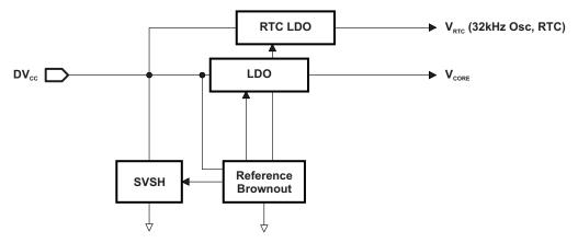
Figure 1. PMM Block Diagram
