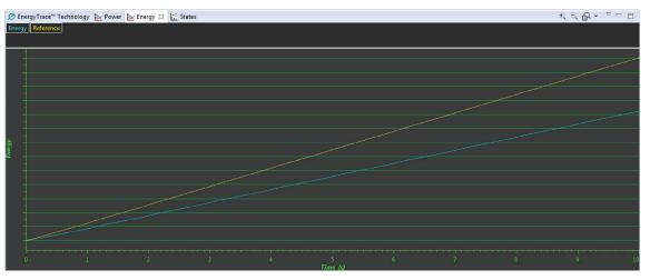
Figure 25. MostEfficient.c Energy (Blue) Referenced With Efficient.c Energy (Yellow)
