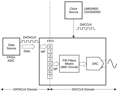
Figure 1. DAC348x Family FIFO Function
