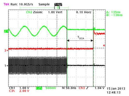
Figure 5. Snapshot of ALARM, DACCLK, and Output Signal of DAC34H84 when DACCLK Is Gone
