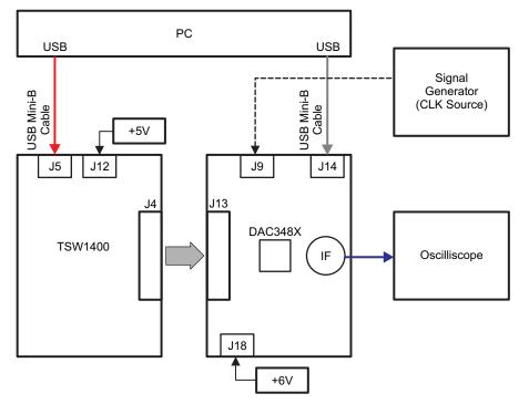
Figure 2. Test Setup Block Diagram for TSW1400 and DAC348x Family
