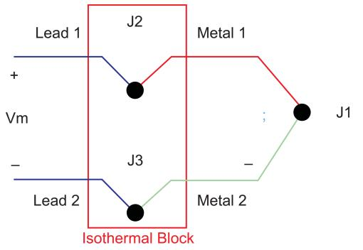
Figure 3. Isothermal Block for Absolute Temperature Measurement
