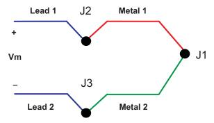
Figure 2. Measuring Thermocouple Voltage with a Voltmeter
