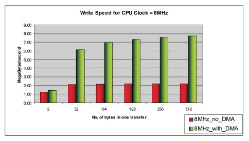
Figure 1. Comparing Write Speeds With and Without DMA Usage
