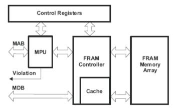
Figure 3. FRAM Controller Block Diagram
