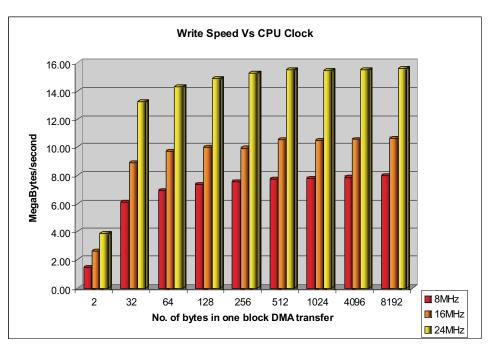
Figure 4. FRAM Write Speed vs. CPU Clock Frequency (MCLK)
