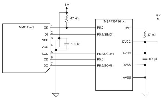
Figure 1. Connection Between MSP430 MCU and MMC Card
