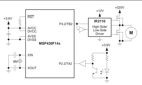
Figure 6. Hardware Block Schematic
