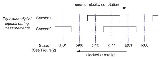
Figure 4. Example Scan IF Signal Digital Representation During Rotation
