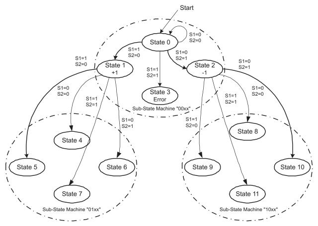
Figure 19. Two-Sensor Transition Detail
