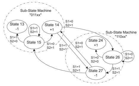
Figure 21. Sensor Bounce Rejection State Transitions
