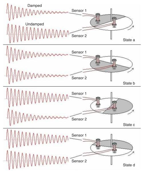
Figure 2. Example LC Sensor Output During Rotation
