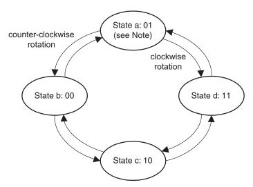
Figure 5. Example State Transitions During Rotation
