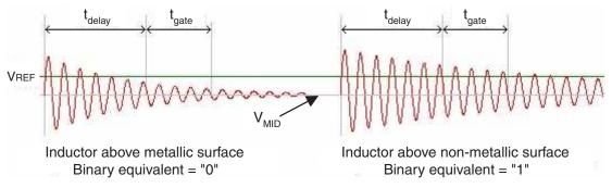
Figure 3. LC Sensor Signal Damping and Scan IF Detection
