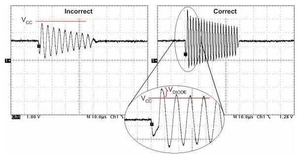
Figure 9. LC Sensor Dimensioning Comparison
