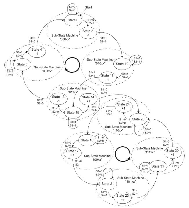
Figure 20. Advanced Two-Sensor PSM with Bounce Reject
