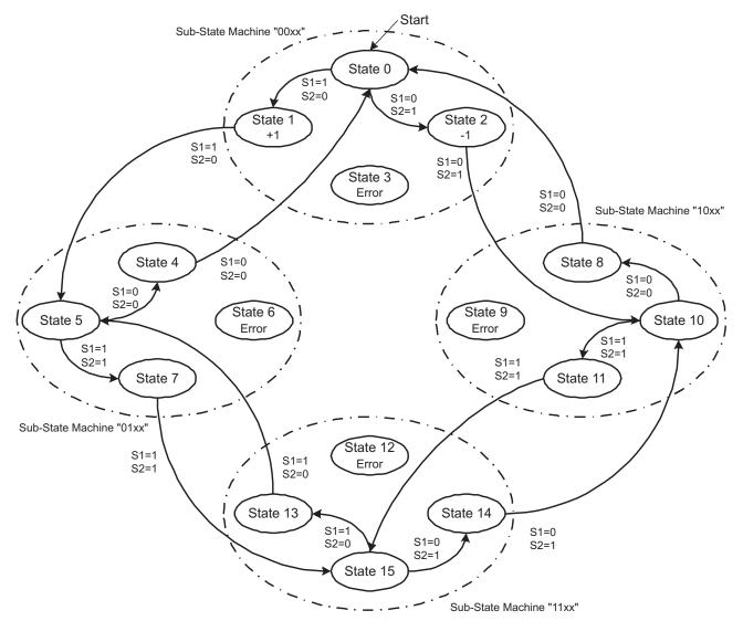
Figure 18. Two-Sensor Simple PSM Example
