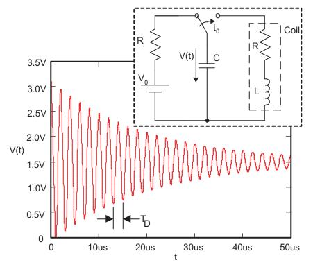
Figure 8. Oscillation Damping of LC Sensor
