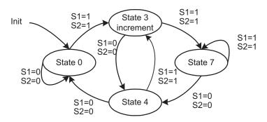
Figure 14. Processing State Machine Example: One Sensor
