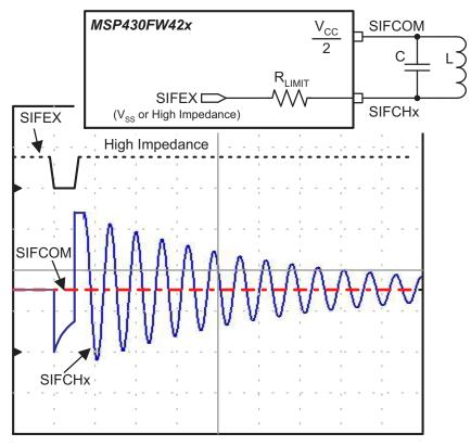
Figure 11. LC Sensor Excitation and Decay Around SIFCOM
