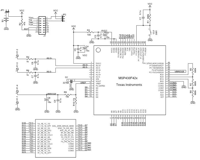
Figure 4. Schematic
