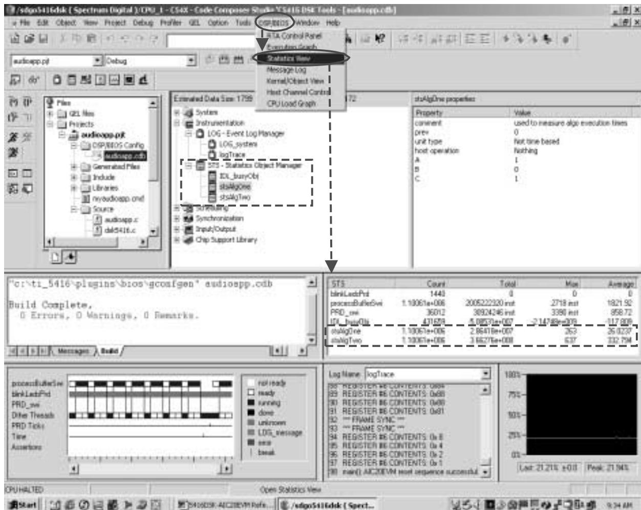
The screenshot shows the CCS IDE interface. The main window displays the DSP/BIOS Statistics View, which is configured to show real-time statistics for STS objects. The Statistics View window is open, showing a tree view of STS objects (stsAlgOne, stsAlgTwo) under the STS - Statistics Object Manager. A table displays real-time statistics for these objects, including Count, Total, Max, and Average. A log window shows the execution of the program, and a CPU load graph is visible at the bottom.
