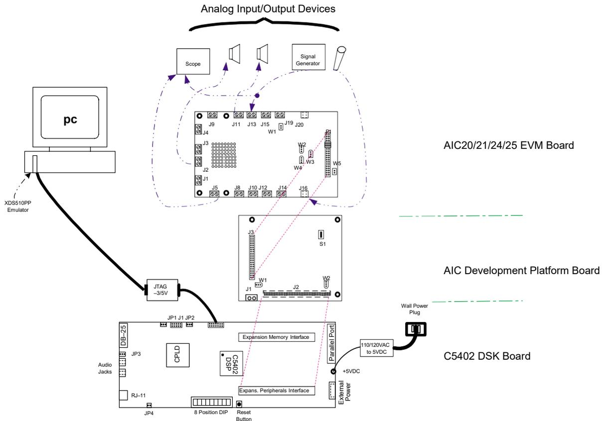
**Figure 1. 2-Device/4-Channel AIC20/21/24/25 EVM System and Hardware Connections**
