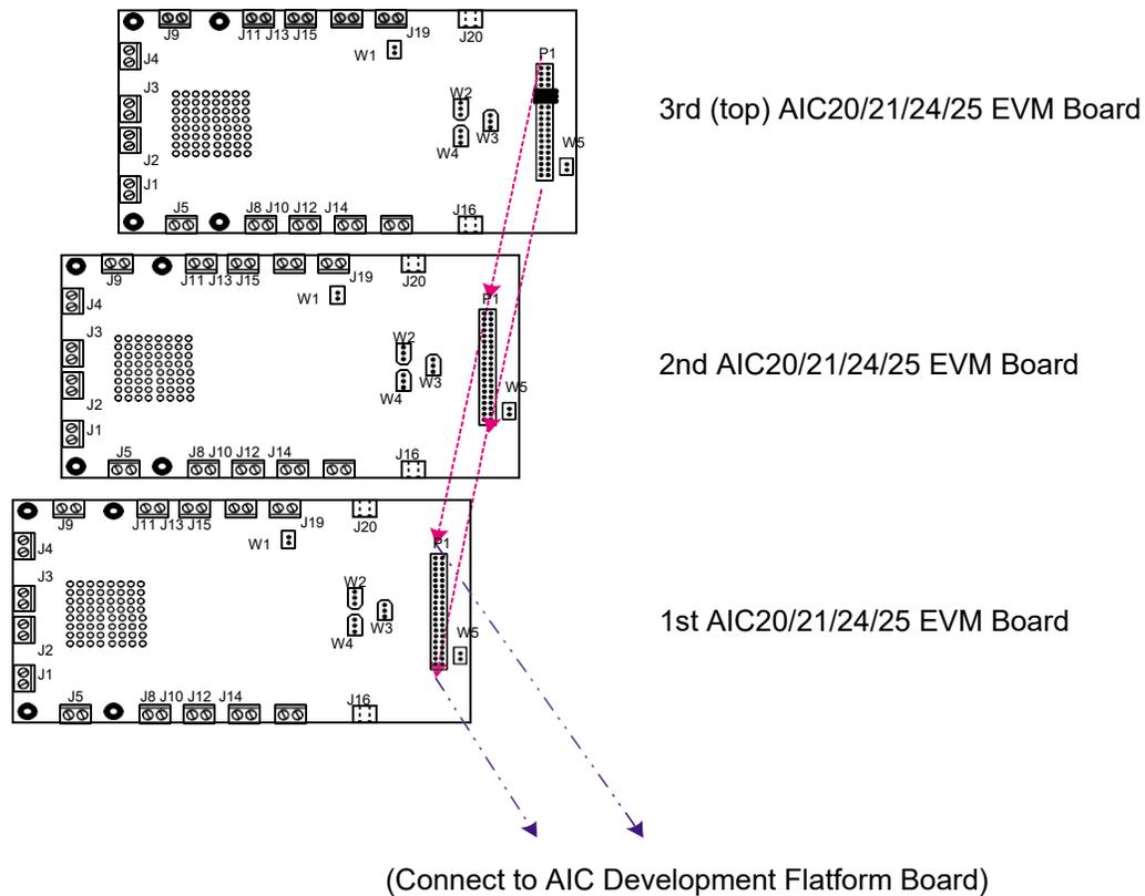
**Figure 2. 6-Device/12-Channel System EVM Boards Connections**
