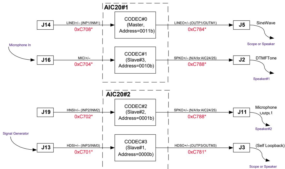
\* The hex code for configuring the corresponding codec control registers.
