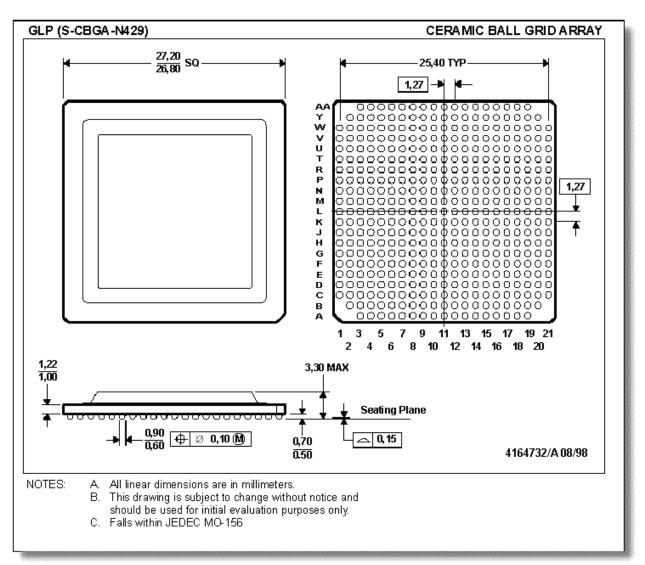
The GLP package is used for the production versions of the ceramic C6X devices: 320C6201B and 320C6701. The C6201BGLP and C6701GLP have identical pinouts and identical footprints.
