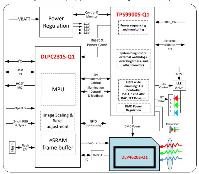
Figure 4-1. DLP4620S-Q1 Chipset Block Diagram
