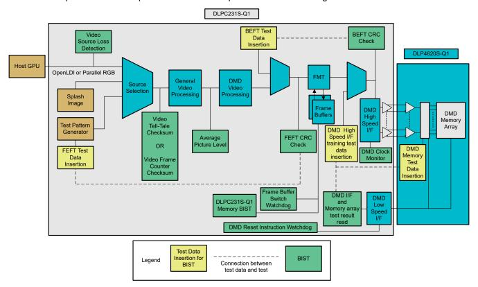
Figure 6-1. DLP4620S-Q1 Video Path With Diagnostics
