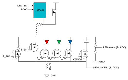
Figure 6-7. LED Driver Architecture
