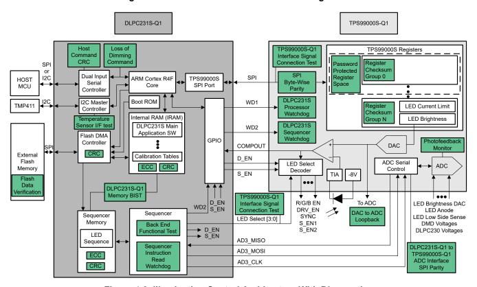
Figure 4-3. Illumination Control Architecture With Diagnostics
