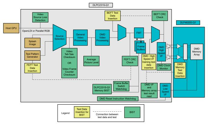
Figure 4-2. DLP4620S-Q1 Video Path With Diagnostics
