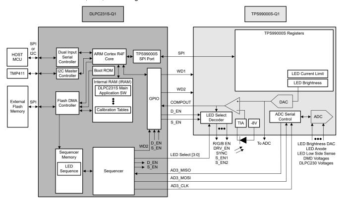
Figure 6-6. Illumination Control Architecture
