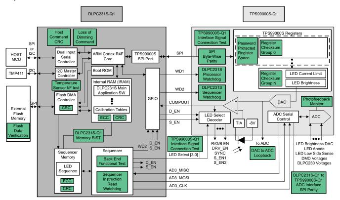
Figure 6-9. Illumination Control Architecture With Diagnostics
