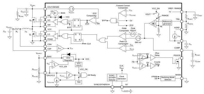
Figure 1-1. Functional Block Diagram
