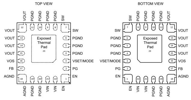
Figure 2-1. Pin Diagram
