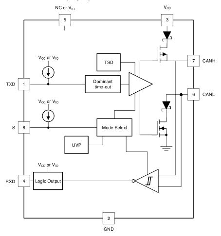
Figure 1-1. TCAN1057A-Q1 and TCAN1057AV-Q1 Functional Block Diagram
