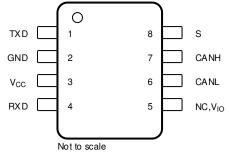
Figure 4-3. D Package, 8-Pin SOIC, Top View
