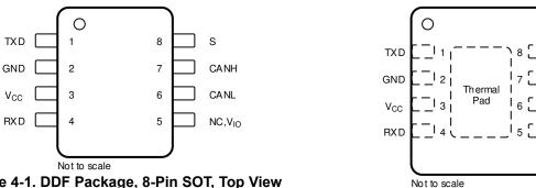
Figure 4-1. DDF Package, 8-Pin SOT, Top View
