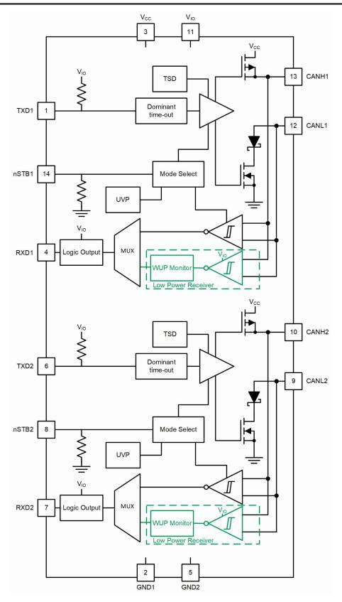
Figure 1-1. TCAN1048AV-Q1 Functional Block Diagram
