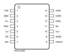
Figure 4-3. SOT Pin Diagram
