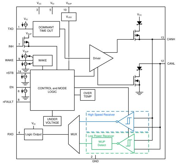
Figure 1-1. TCAN1043A-Q1 Functional Block Diagram
