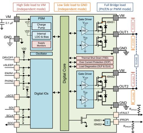
Figure 1-3. Functional Block Diagram for SPI "P" variant
