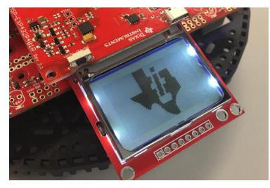
Microcontrollers employ multiple approaches to communicate synchronously with peripheral devices and other microcontrollers. The synchronous peripheral interface (SPI) system can operate as a master or as a slave. The channel can have one master and one slave, or it can have one master and multiple slaves. In this module, the MSP432 will be the master and the LCD will be the slave. The master initiates all data communication.
