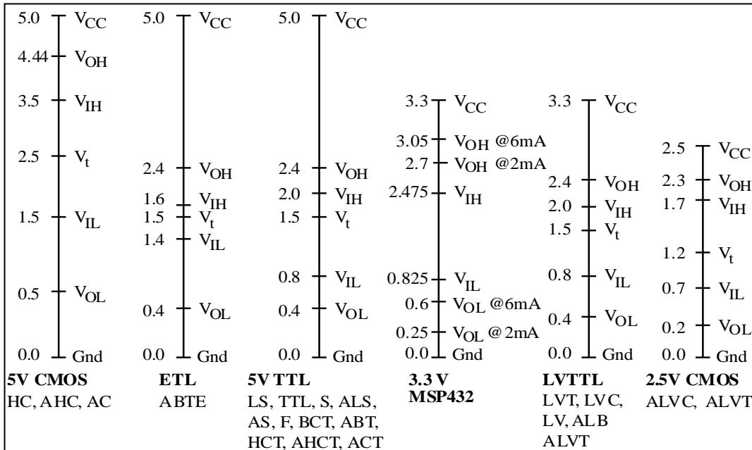
$V_{OL} \leq V_{IL}$  for all inputs    and     $V_{OH} \geq V_{IH}$  for all inputs
