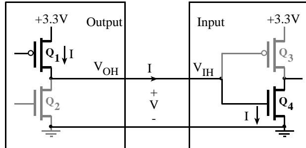
$V_{OL} \leq V_{IL}$  for all inputs and  $V_{OH} \geq V_{IH}$  for all inputs
